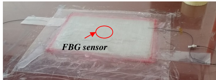
Figure 4: Composite sample was cured for 24 hours in room temperature, and atmospheric pressure.
