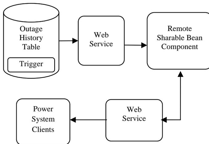
Fig. 1 Block Diagram Representation of the Event Notification System
