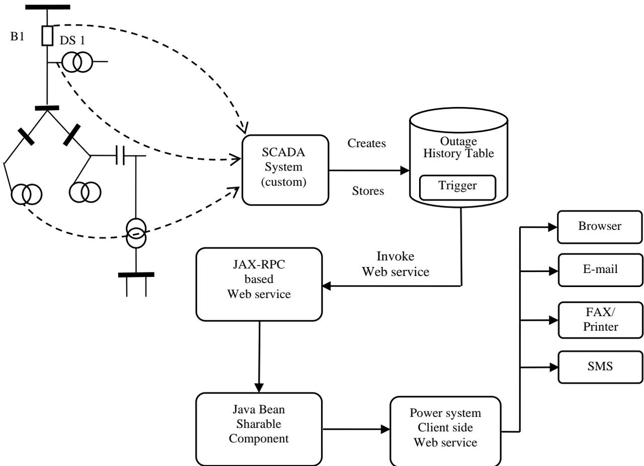
Fig. 2 Secure and Reliable Synchronized Event Notification System
