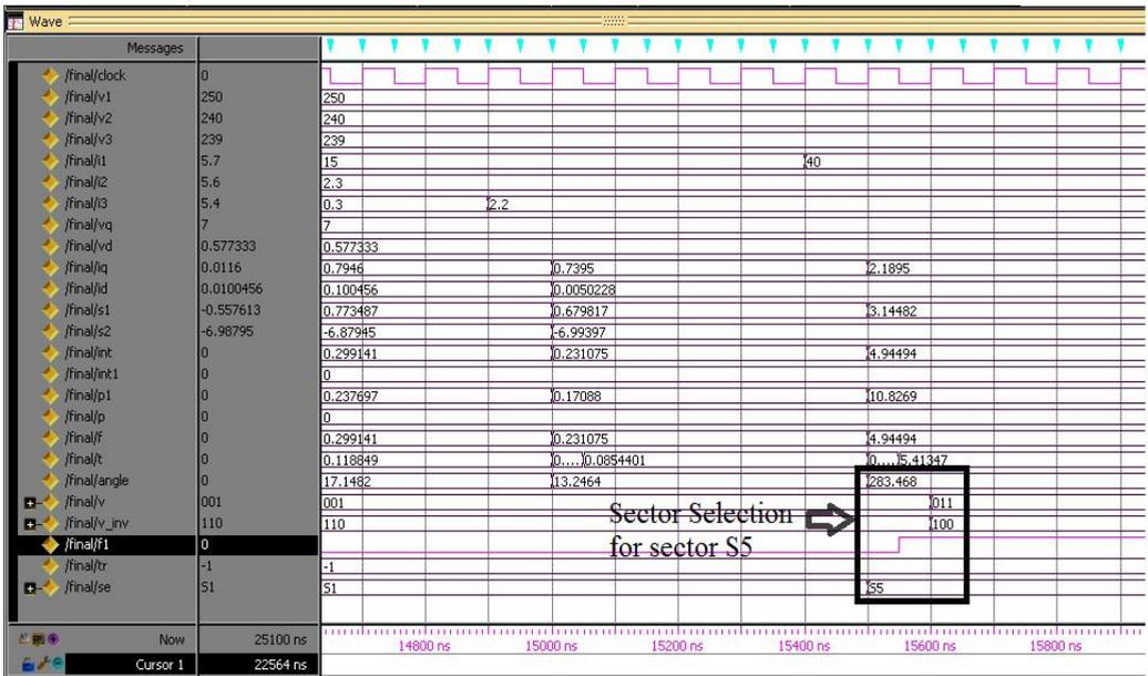
Figure 10 (c) Simulation results showing the sector selection S5 for an angle 283.4 ( $240 < \alpha < 300$ )
