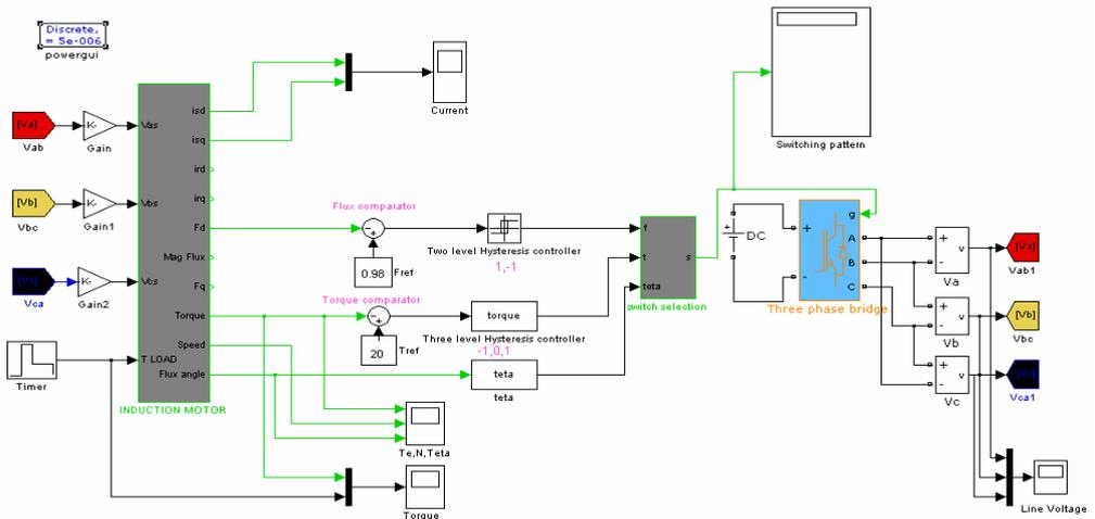
Figure 4 Simulink Model of Space Vector Modulation based Direct Torque Control
