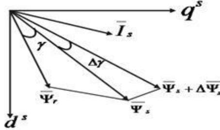
Figure 3 Stator flux and rotor flux space vectors
