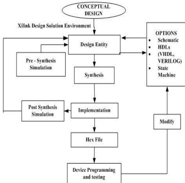
Figure 9 VHDL Programming Design Flow
