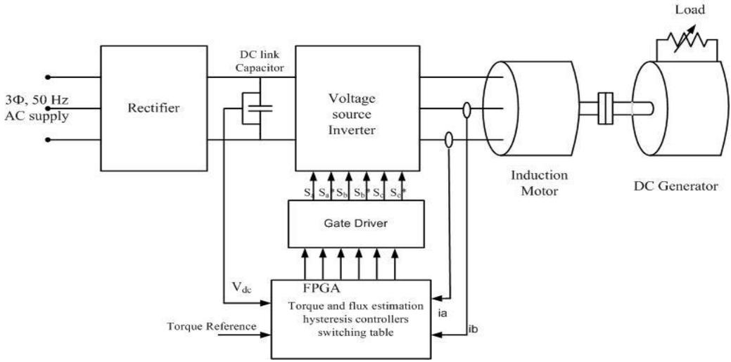
Figure 10(a) Functional Block diagram of SVM based DTC using FPGA circuits
