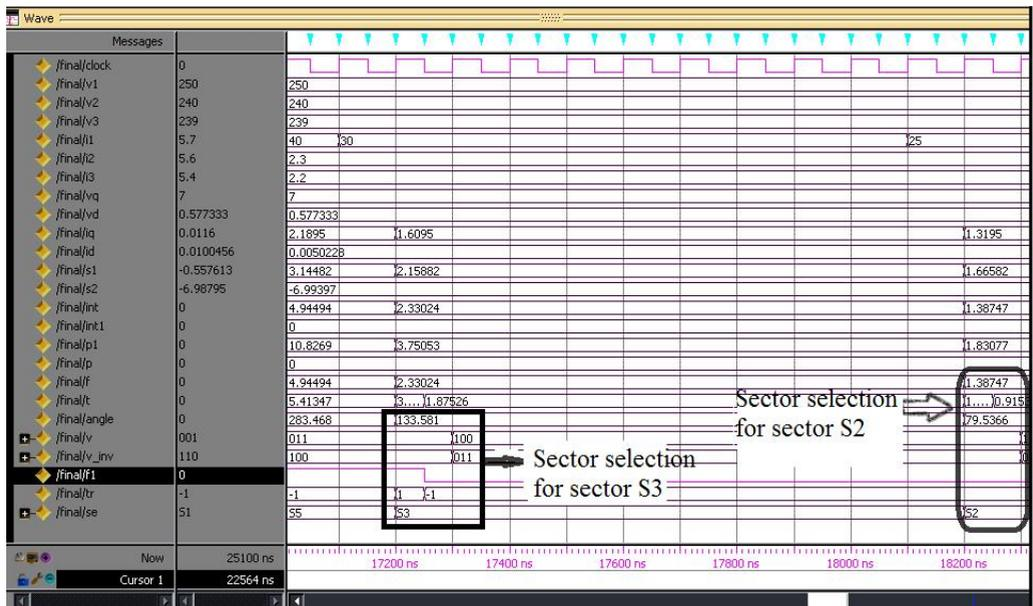
Figure 10(b) Simulation results showing the sector selection S2 for an
