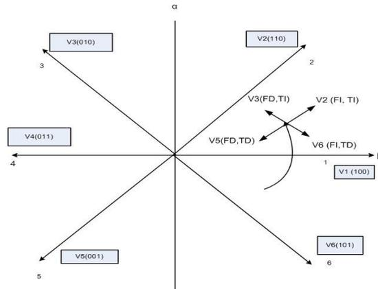
Figure 2 Stator flux vector locus and different possible switching voltage vectors. FD: flux decrease, FI: flux increase, TD: torque decrease, TI: torque increase.
