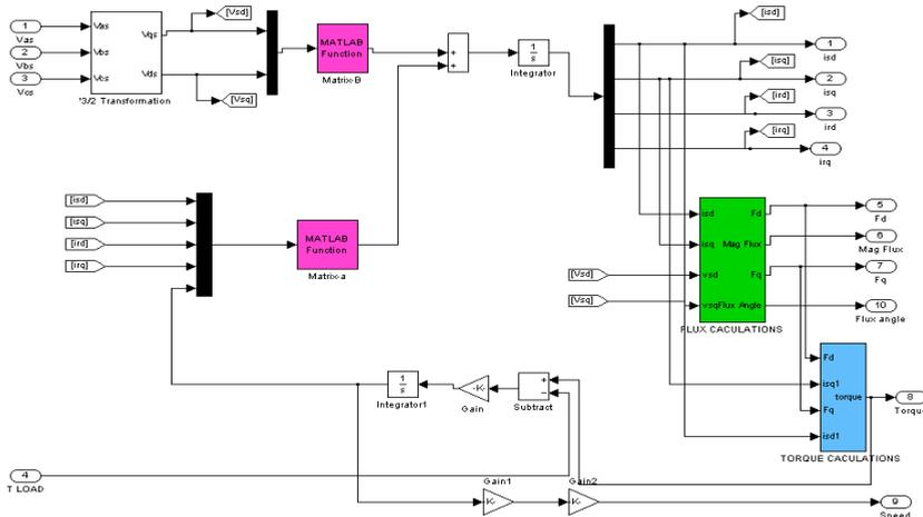
Figure 5 Simulink Model of Induction Machine
