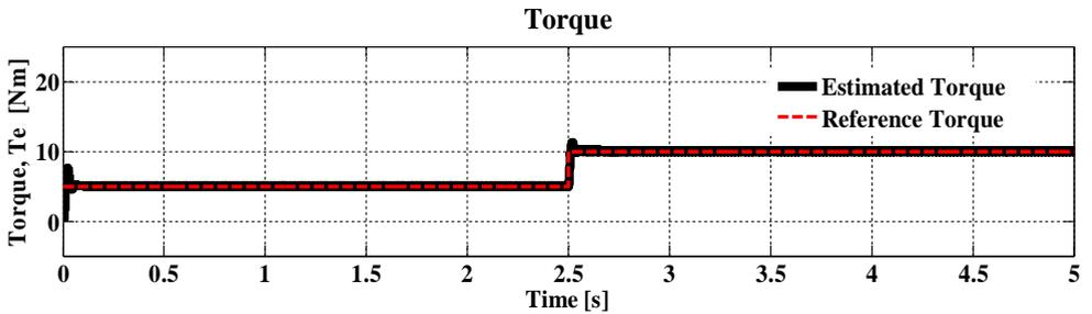
Figure 7 Simulation results of Electromagnetic Torque
