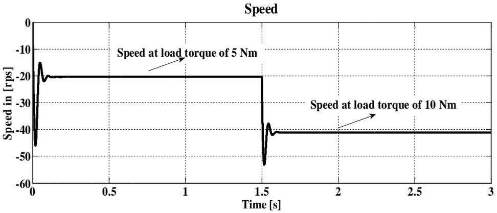
Figure 8 Simulation results of motor speed response
