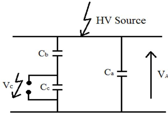
Fig.1 Sample model with void.
