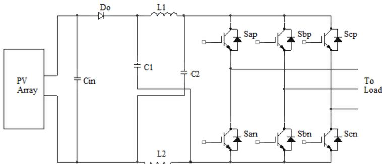
Fig.1. Z-source inverter
