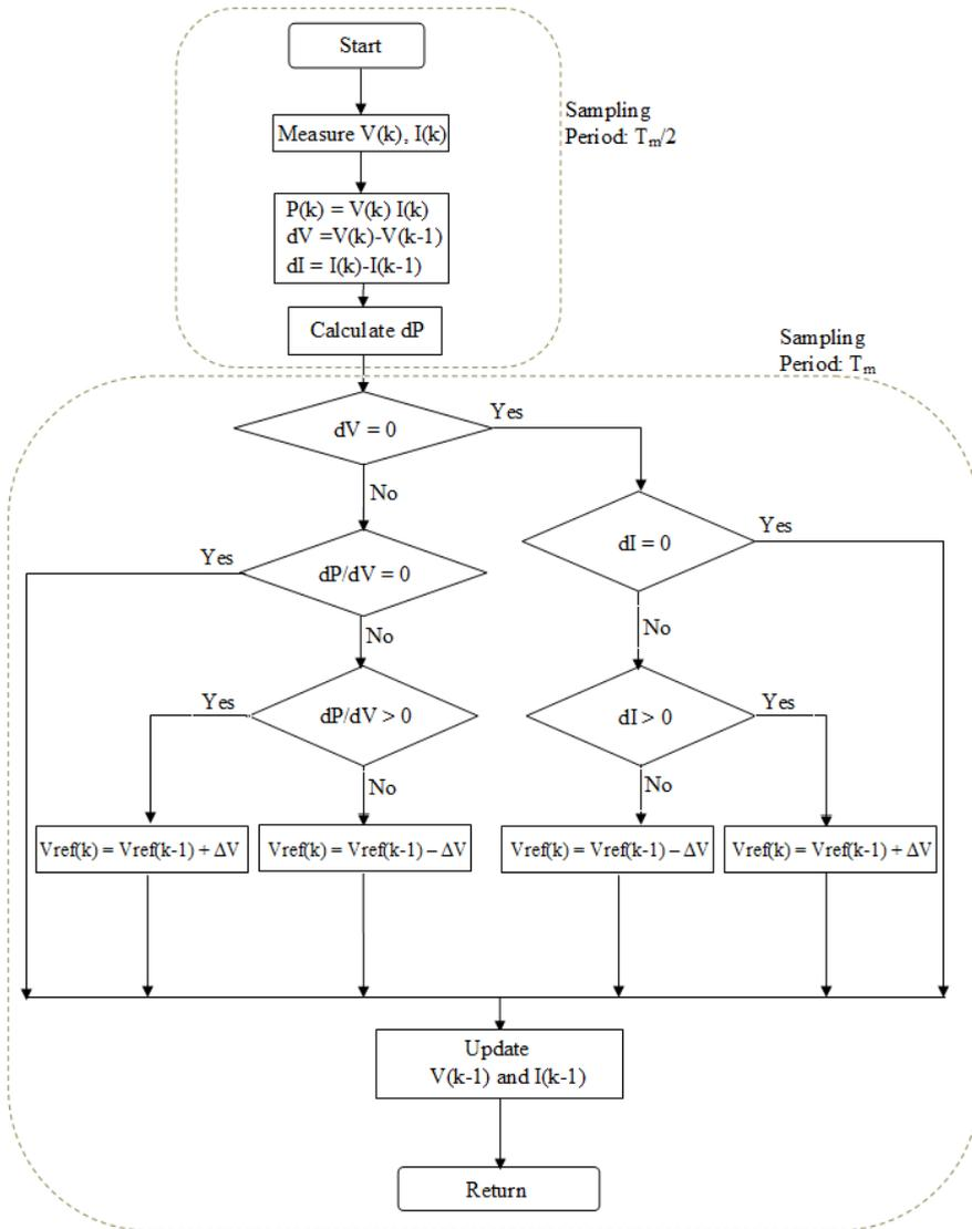
Fig. 4. Flow chart of modified incremental conductance algorithm
