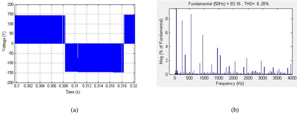
Fig.7. Simulation results (a) Output line voltage (b) Harmonic spectrum of output line voltage
