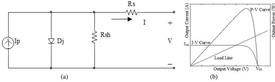
Fig.2. Photovoltaic cell (a) Equivalent circuit (b) Typical I-V and P-V characteristics
