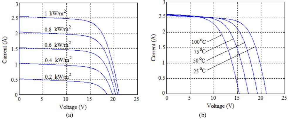
Fig.5. I-V output characteristics of PV module with different (a) solar irradiation (b) temperature
