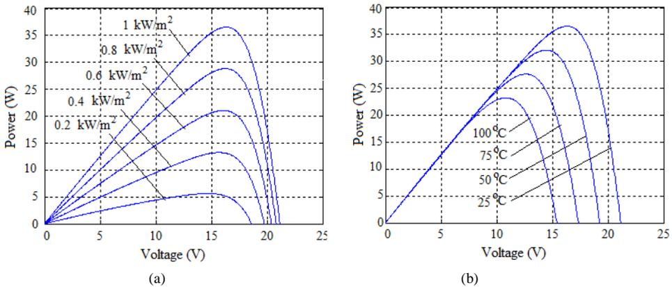
Fig.6. P-V output characteristics of PV module with different (a) solar irradiation (b) temperature
