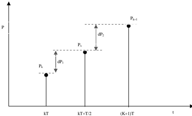
Fig. 3.Measurement of Power between two sampling instances
