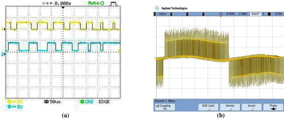
Fig.8. Experimental Waveforms (a) Switching pulses (b) Output line voltage waveform
