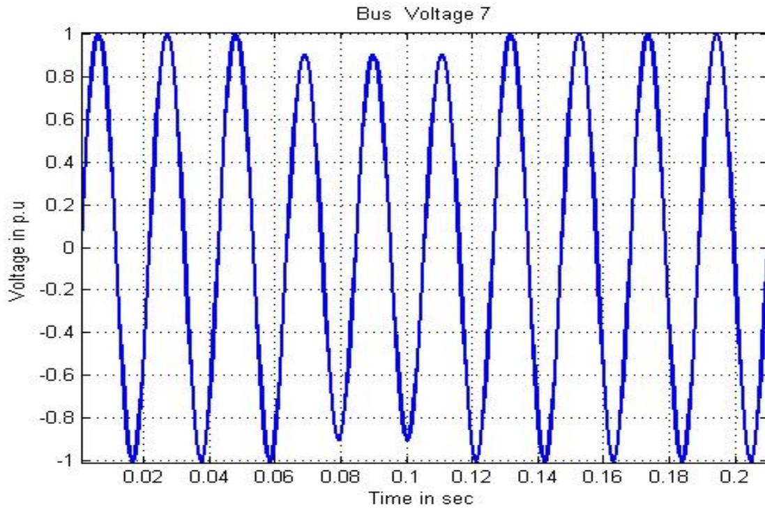
Figure 6: The performance of the 7<sup>th</sup> bus voltage for one DG connection
