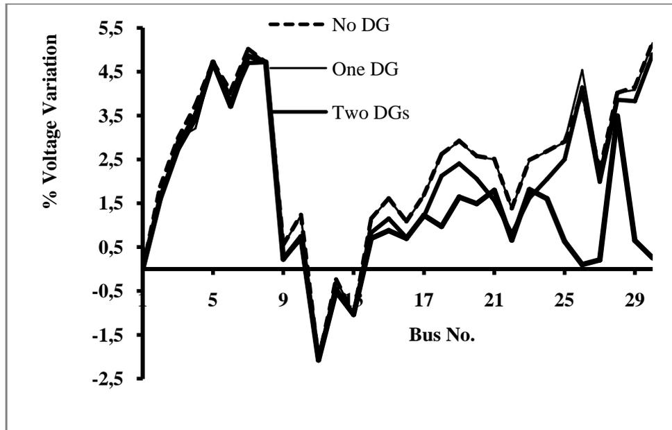
Figure 18: Percentage Variations of Bus Voltages Compared with Slack Bus Voltage
