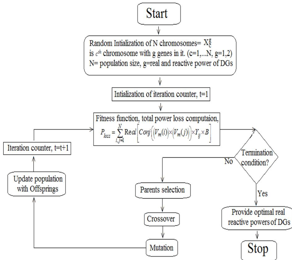
Figure 2: Flow chart of GA for providing DGs optimal real and reactive powers
