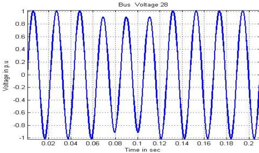
Figure 9: The performance of the 28<sup>th</sup> bus voltage for one DG connection
