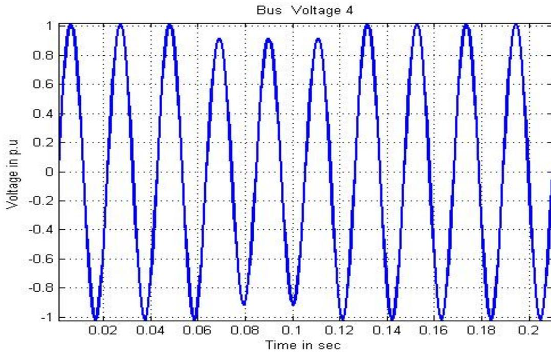
Figure 4: The performance of the 4<sup>th</sup> bus voltage for one DG connection
