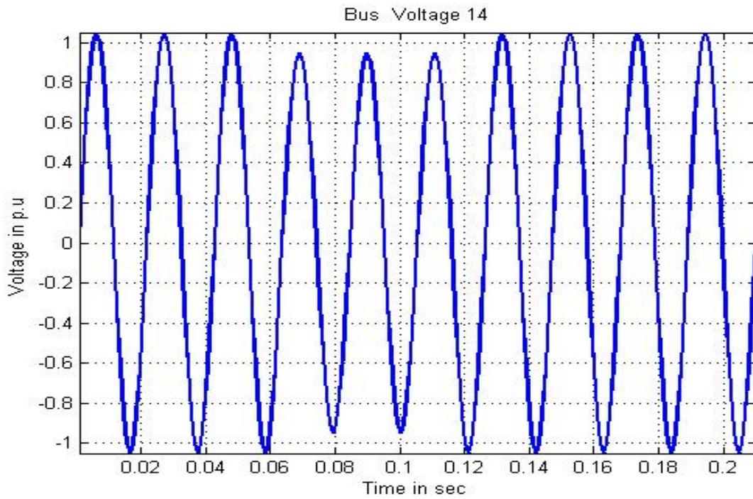
Figure 13: The performance of the 14<sup>th</sup> bus voltage for 2 DG connection
