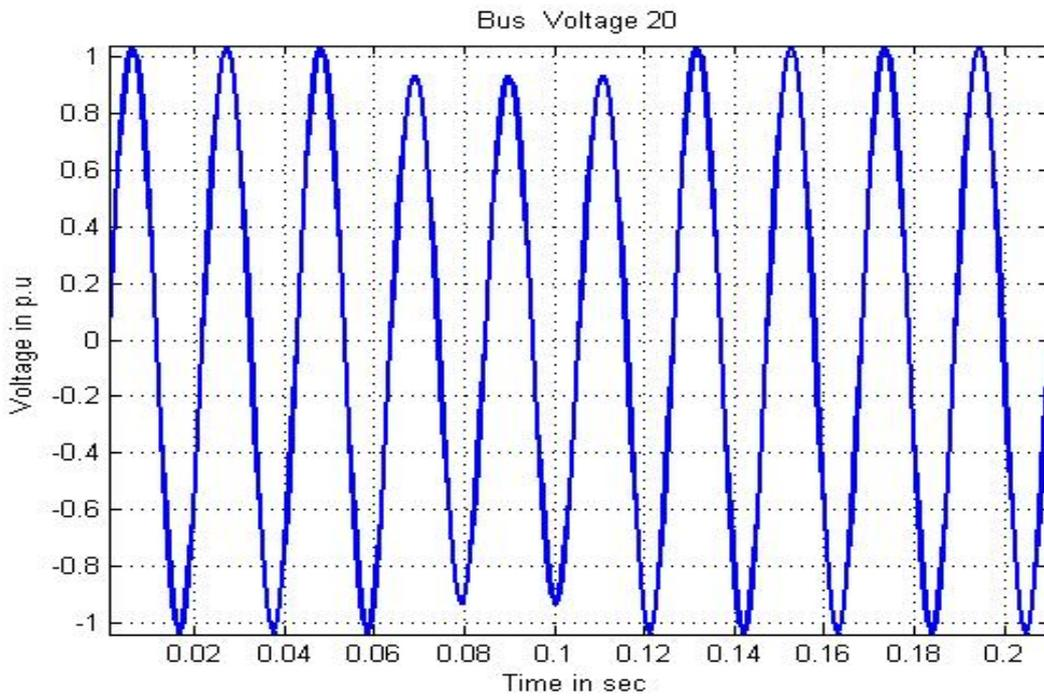
Figure 15: The performance of the 20<sup>th</sup> bus voltage for 2 DG connection
