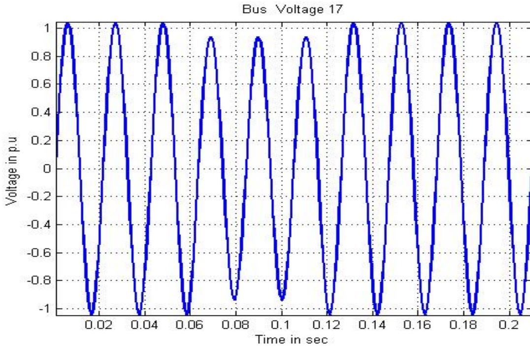
Figure 14: The performance of the 17<sup>th</sup> bus voltage for 2 DG connection
