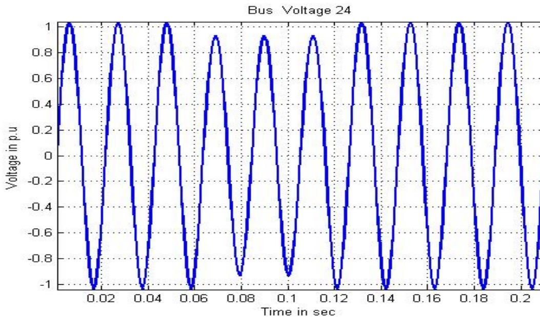
Figure 16: The performance of the 24<sup>th</sup> bus voltage for 2 DG connection
