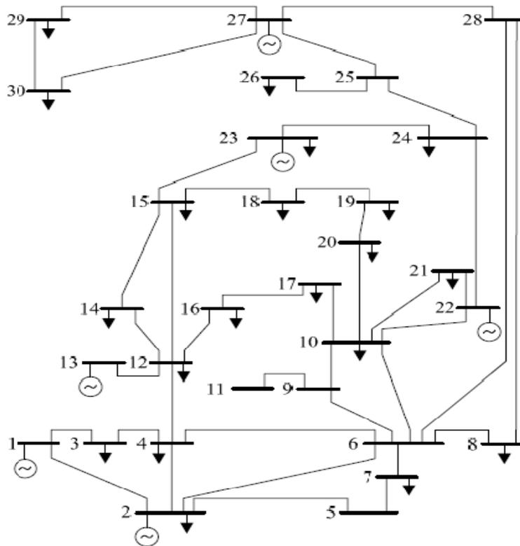
Figure 3: IEEE 30 Bus test system
