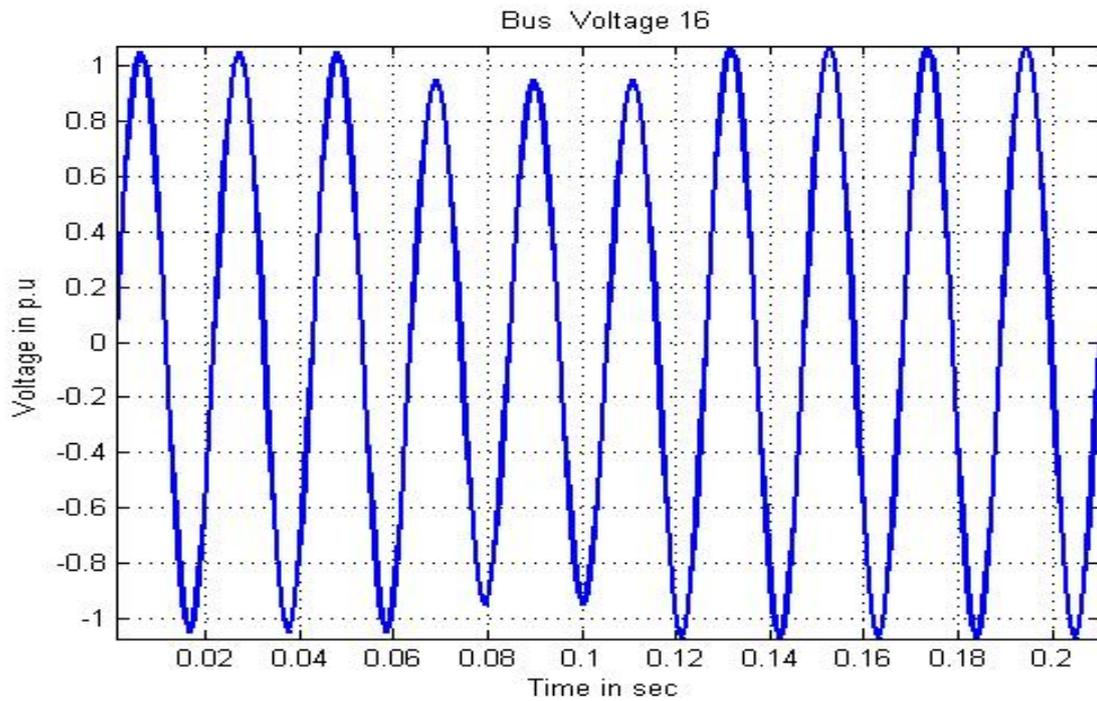
Figure 7: The performance of the 16<sup>th</sup> bus voltage for one DG connection
