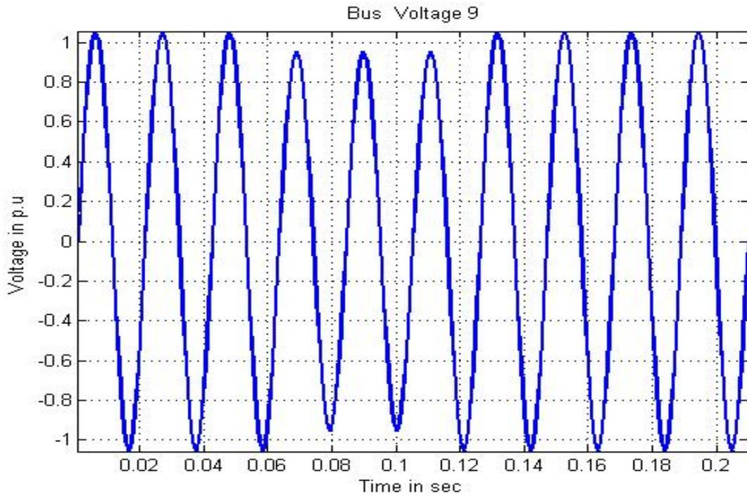
Figure 12: The performance of the 9<sup>th</sup> bus voltage for 2 DG connection
