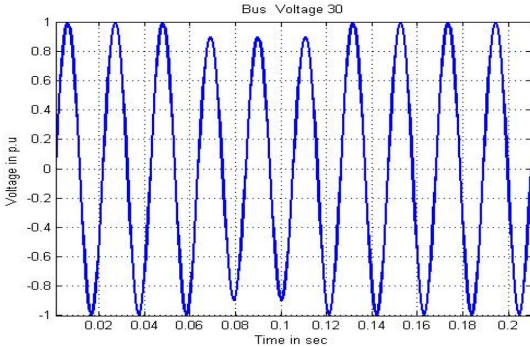
Figure 10: The performance of the 30<sup>th</sup> bus voltage for one DG connection
