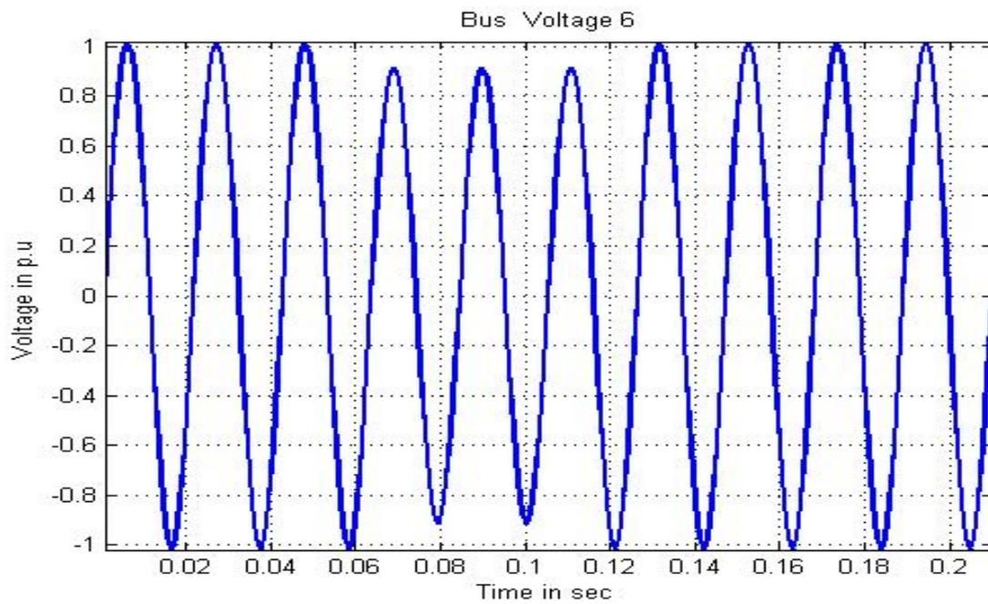
Figure 5: The performance of the 6<sup>th</sup> bus voltage for one DG connection
