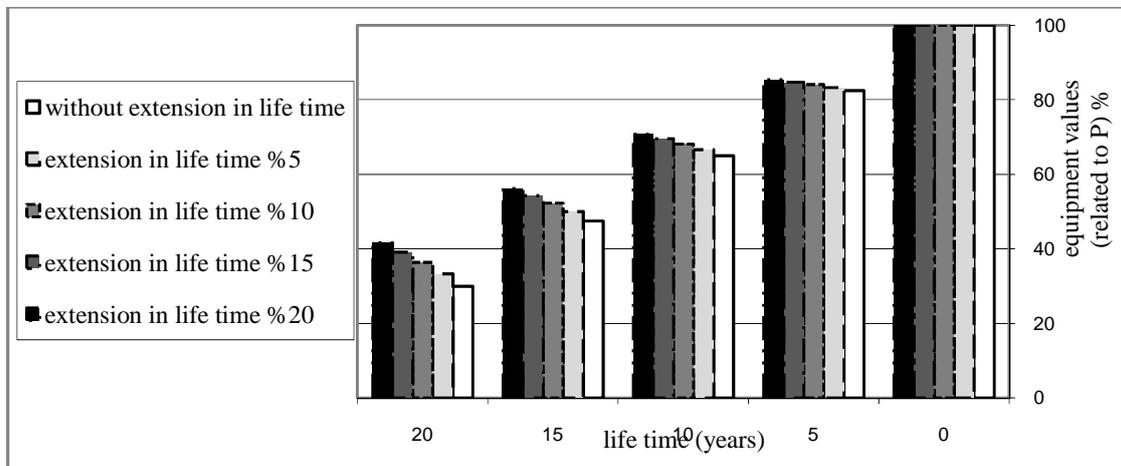
Fig. 3 Increase of Equipment values due to inspection at different equipment lifetime
