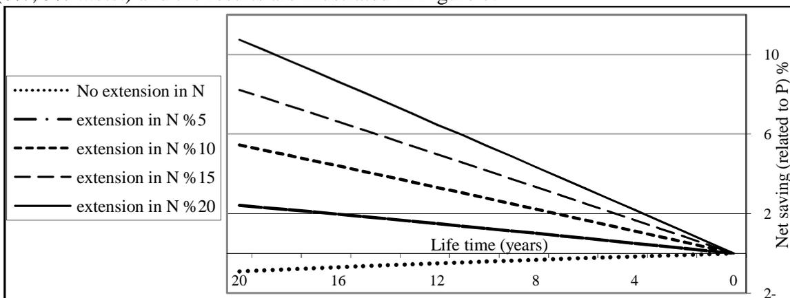
Fig. 7 Net saving (return due to extended lifetime - internal accumulated inspection costs)
