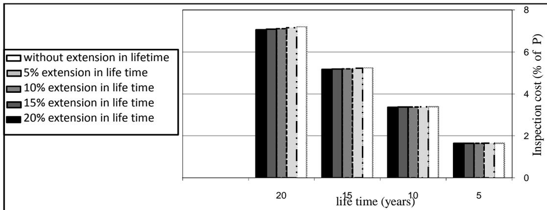
Fig. 4 Inspection costs during equipment lifetime: External inspection
