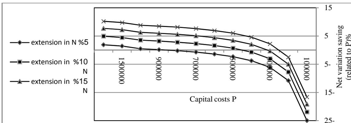
Fig. 8 Variation of saving due to inspection with the capital cost for different values of extension lifetime
