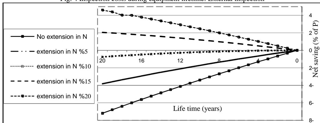
Fig. 5 Net Saving (Return due to extended lifetime - External accumulated inspection costs)
