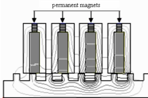
Fig.7. New reluctant polarized structure
