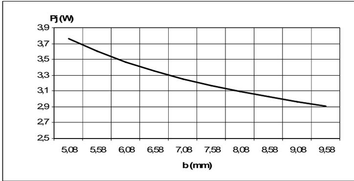
Fig.3. Joule losses as a function of slit width ‘b’
