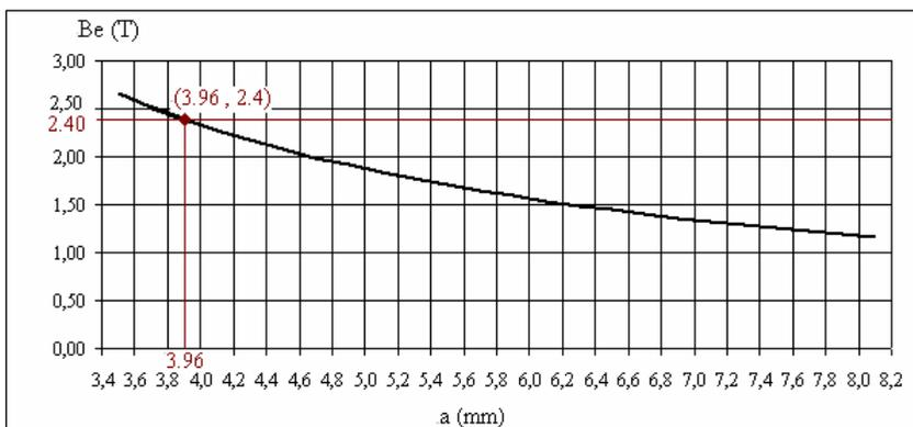
Fig.6. Induction airgap values according to the tooth width
