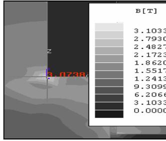
Fig.13. Induction saturation in the corner slit ( $B=3T$ )
