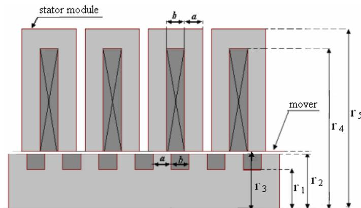
Fig.2. Geometrical parameters of the existing motor
