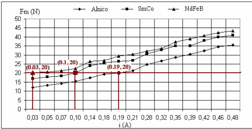
Fig. 8. Maximal force as a function of the current  $i$
