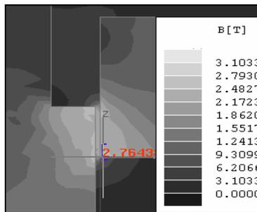
Fig.11. Saturation in tooth extremities ( $B=2.76T$ )
