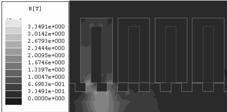
Fig.5. Induction in a magnetic module for  $a=b=5.08\text{mm}$
