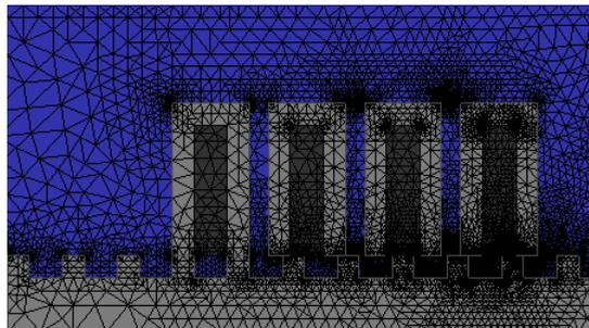
Fig.4. Finite elements model of the studied stepping motor
