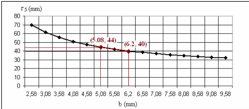
Fig.9. Exterior radius  $r_5$  as a function of slit width “b”
