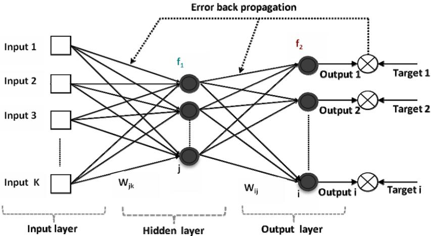
Figure 2: Schematic diagram of a multilayer feed forward ANN
