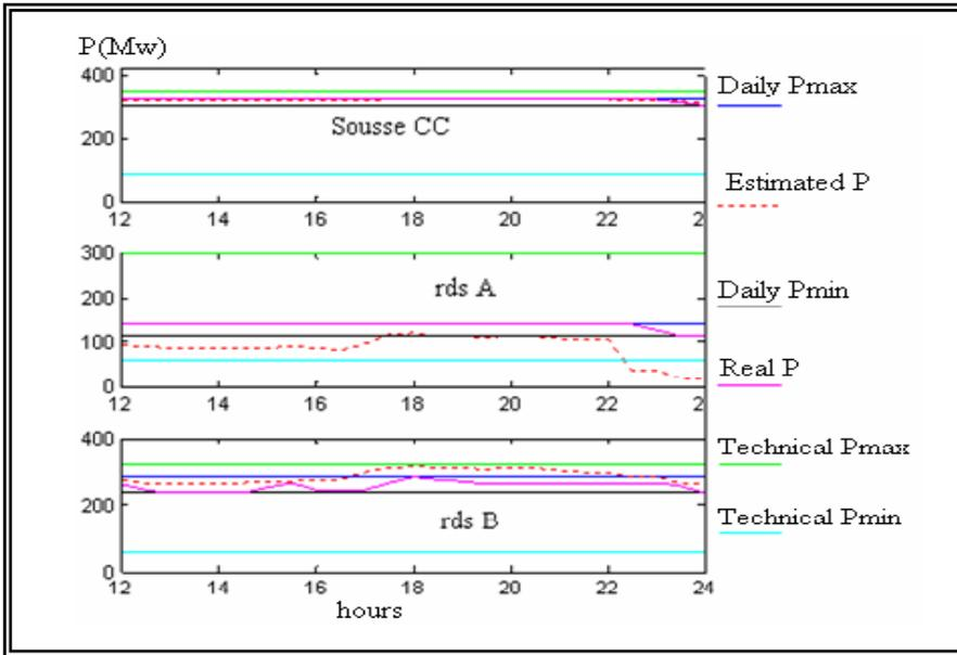
Figure 12: Power produced by each basic plant (sousseCC, rdsA, rdsB)
