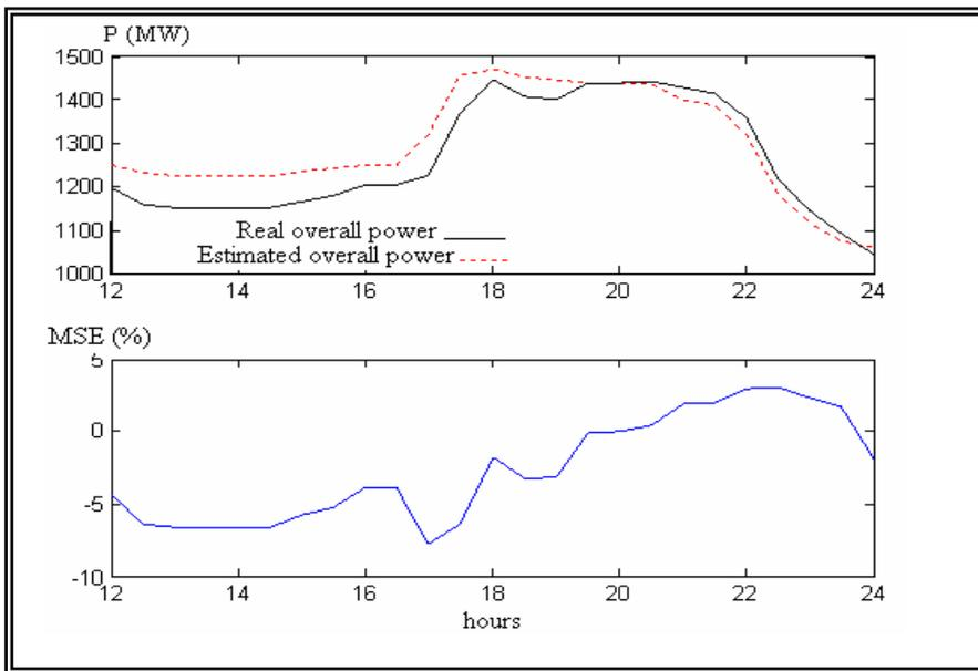
Figure 10: Total real and estimated power following the integration of intermittent  $P_{wind}$ : 2<sup>nd</sup> period
