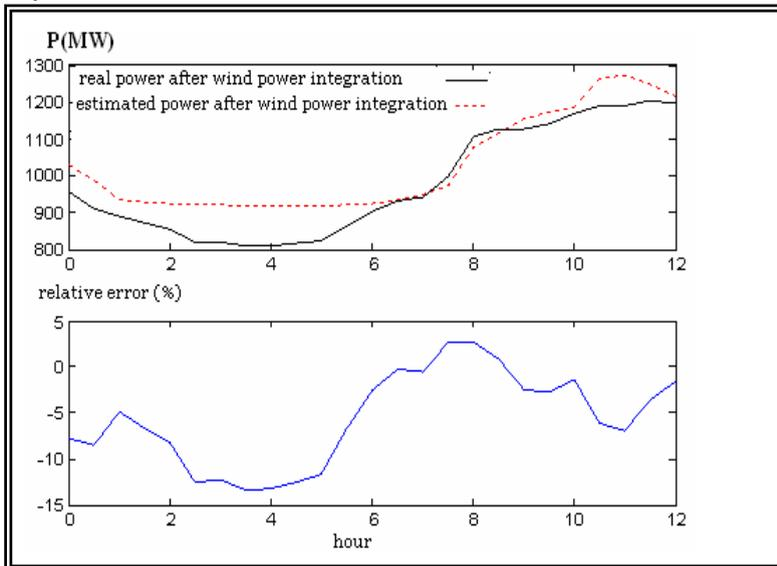
Figure 6: Comparison between real and estimated power after wind power integration
