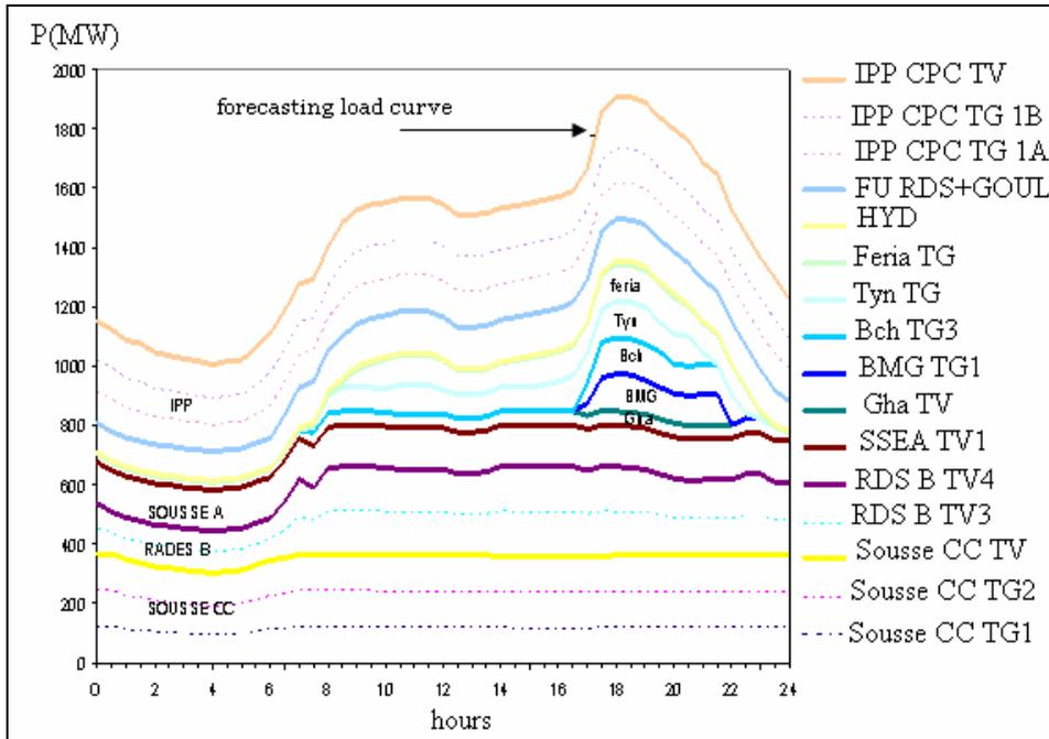
Figure 1: Distribution of the consumption for an ordinary day (T: turbine, V: steam, G: gas, CC: Combined Cycle)
