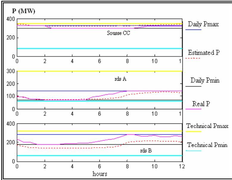
Figure 7: Power produced by (sousseCC, rdsA, rdsB) before and after wind power integration
