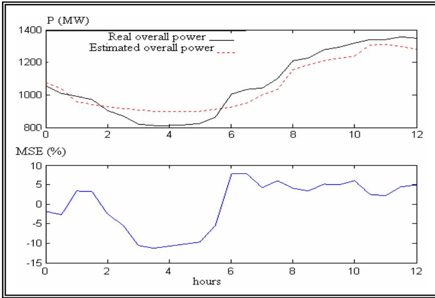
Figure 9: Total real and estimated power following the integration of intermittent  $P_{wind}$ : 1<sup>st</sup> period
