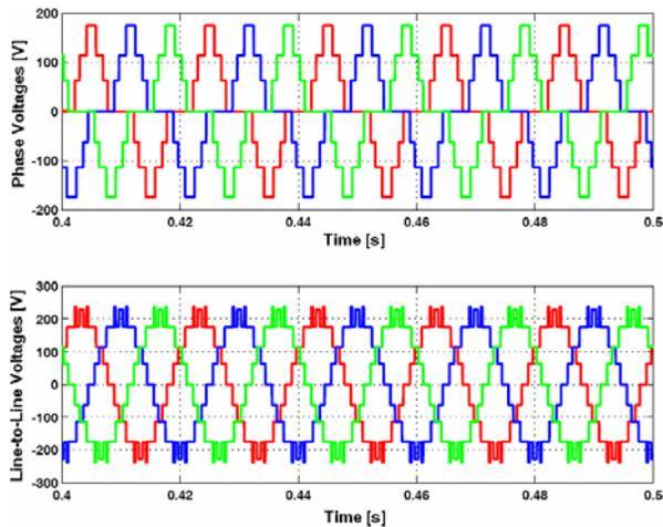
Fig. 4. Phase and line to line voltage waveforms for *m*=0.52.
