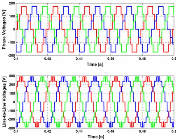
Fig. 9. Phase and line to line voltage waveforms for  $m=0.70$
