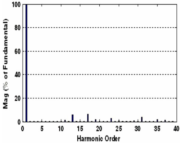
Fig. 11. Normalized FFT of the line to line voltage between phases *a* and *b* shown in Fig. 9.
