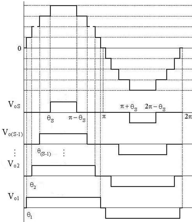
Fig. 2. Waveforms showing the cascaded multi-level inverter output phase voltage and each H-bridge output voltage.
