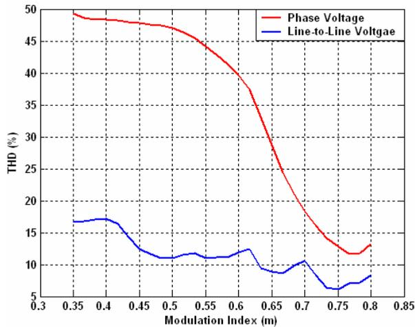
Fig. 12. The phase and line to line output voltage THD of a 7-level inverter as a function of  $m$
