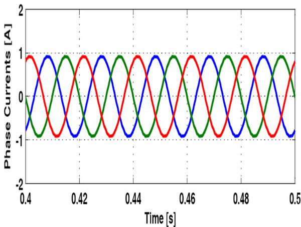
Fig. 7. Output current waveforms for  $m=0.52$ .
