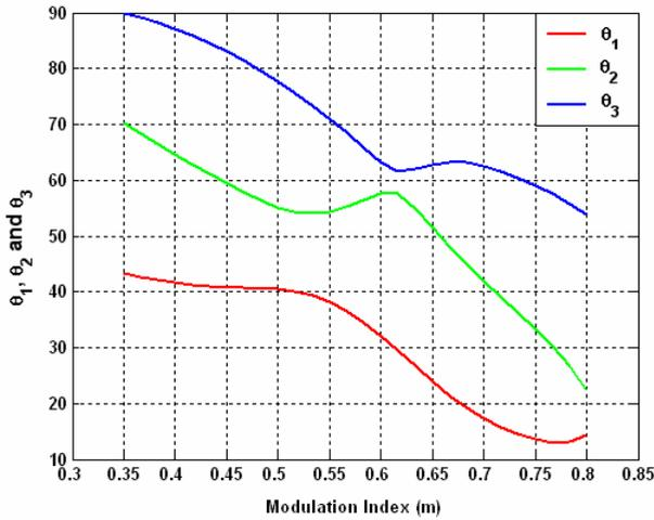
Fig. 3. Switching angles versus *m*.
