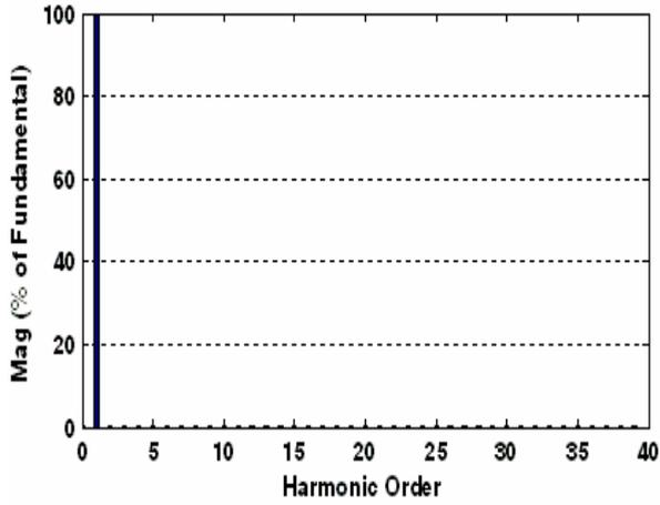
Fig. 8. Normalized FFT of the phase *a* current waveform shown in Fig. 7.
