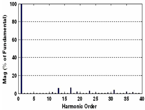
Fig. 6. Normalized FFT of the line to line voltage between phases *a* and *b* shown in Fig. 5.
