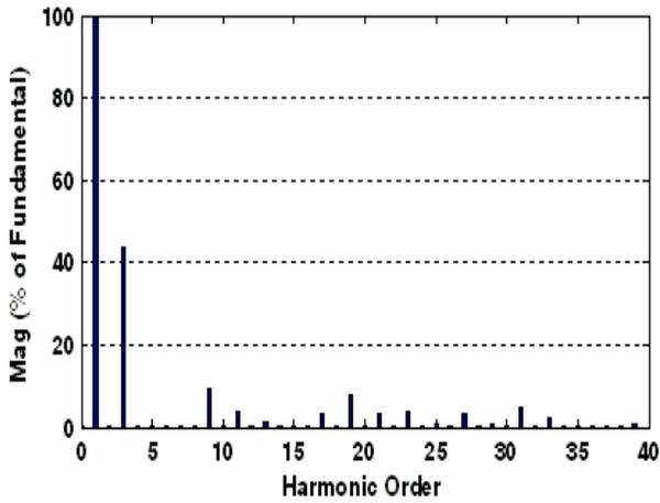
Fig. 5. Normalized FFT of the phase *a* voltage waveform shown in Fig. 5.
