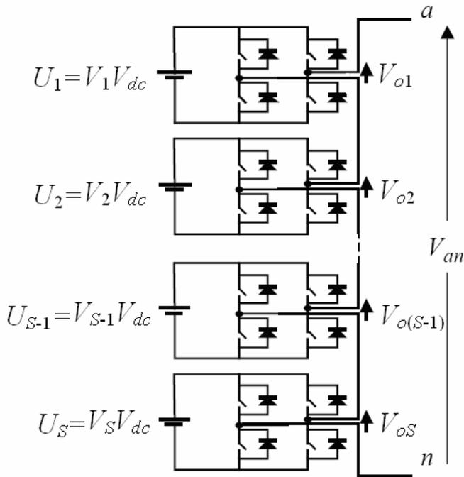
Fig. 1. Single-phase structure of a cascaded H-Bridge multi-level inverter with *unequal* DC sources.
