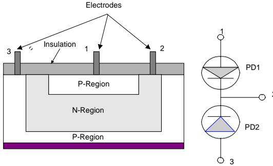
Figure 6. Sharp PD150 sequential photodiode
