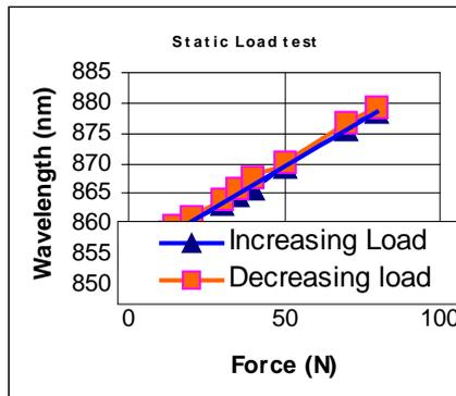
Figure 8. Response of the Strain Gauge to a static Load.
