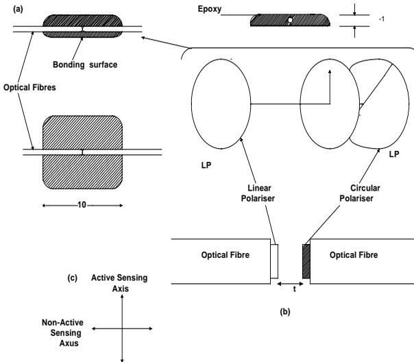
Figure 4. Configuration of: (a) casting unit (b) active element detail (c) sensing axes.
