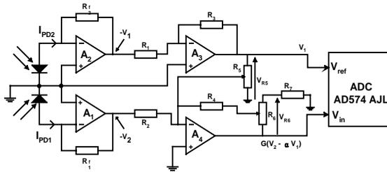
Figure 7. Schematic of the Processing Circuit.
