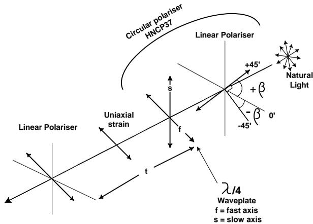
Figure 5. Optical Arrangement showing the Angle  $\beta$  for Crossed Linear / Circular Polariser Arrangement.
