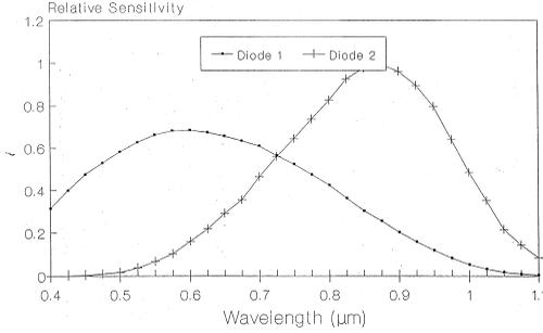
Figure 2. The spectral sensitivities of the overlapping photodiodes
