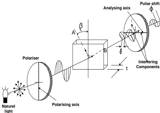
Figure 1. Polarised Light Propagating through Stressed Plastics
