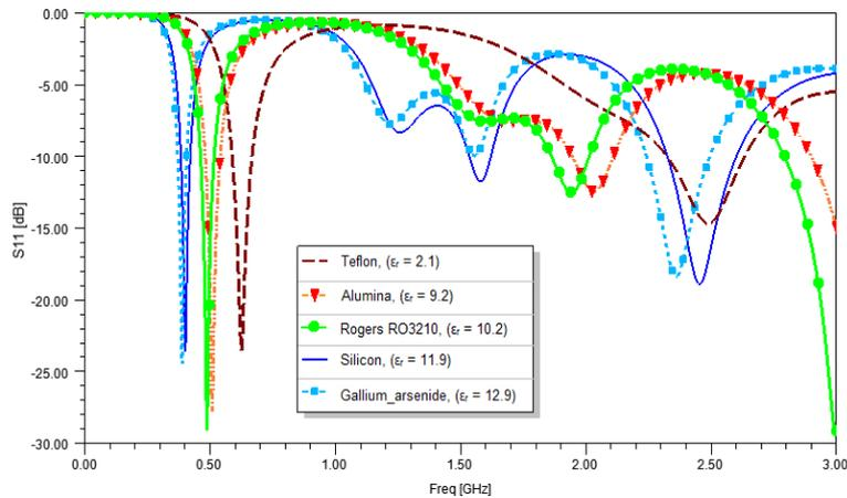
Figure 9 : Simulated return loss S11 for different dielectric materials.
