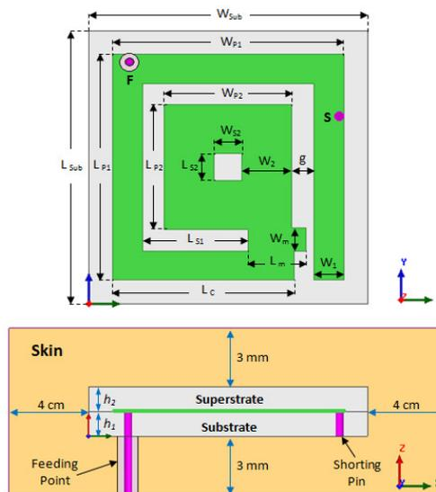
Figure 2 : Proposed antenna geometry.
