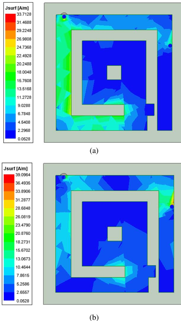
Figure 11 : The electric field distribution, (a) at 403 MHz, (b) at 2.45 GHz.
