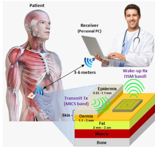
Figure 1 : A block diagram of an implant biomedical monitor system.
