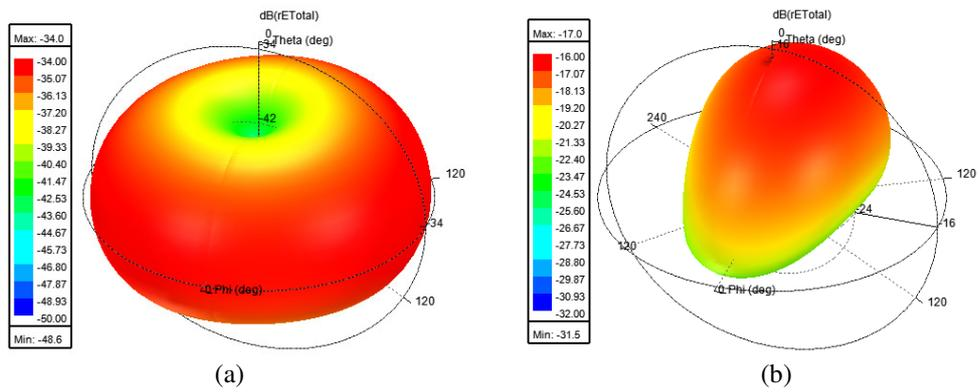
Figure 7 : 3D radiation patterns of the proposed antenna, (a) at 403 MHz, (b) at 2.45 GHz.
