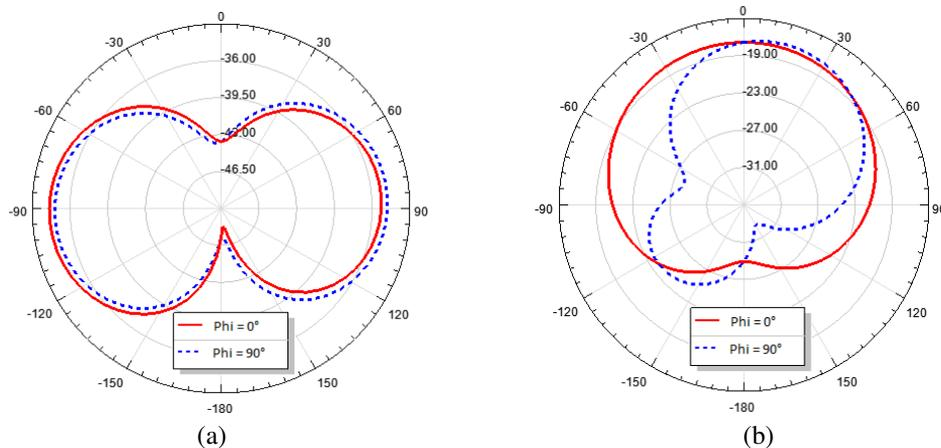
Figure 6 : 2D radiation patterns of the proposed antenna in the E-plane and H-plane, (a) at 403 MHz, (b) at 2.45GHz.
