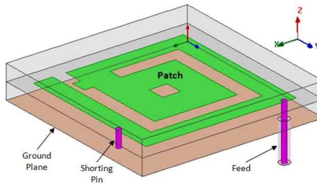
Figure 4 : 3D model view of the proposed antenna.
