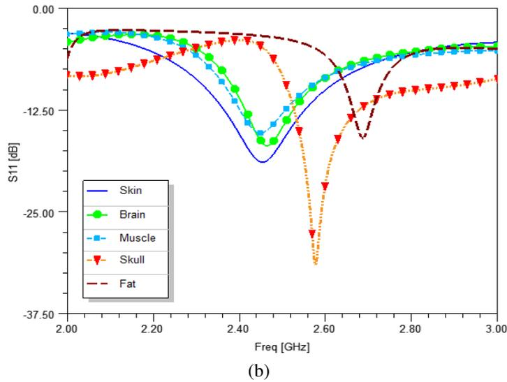
Figure 8 : Simulated return loss S11 for different human body tissues, (a) In MICS band, (b) In ISM band.
