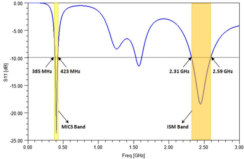
Figure 5 : Simulated return loss S11 of the proposed antenna.
