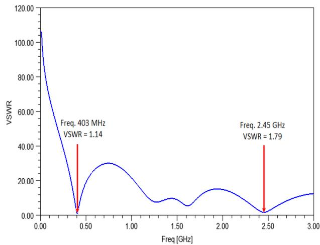
Figure 10 : VSWR for two resonating frequencies in MICS and ISM bands.
