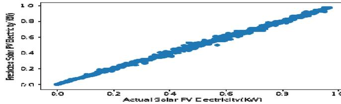
Fig. 9: Forecasting of solar PV electricity by applying decision tree algorithm
