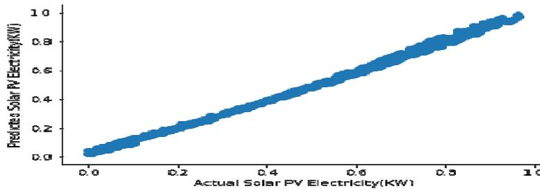
Fig.7: Forecasting of solar PV electricity by applying ridge regression
