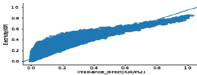
Fig. 2: Regression plot between solar PV electricity and irradiance direct
