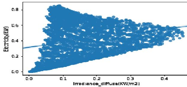
Fig. 3: Regression plot between solar PV electricity and irradiance diffuse
