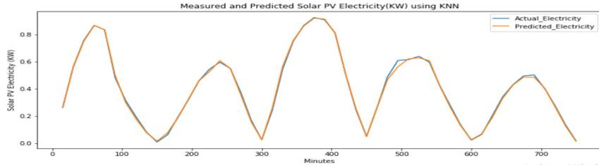
Fig. 23: Solar PV electricity versus time by applying KNN
