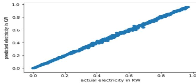
Fig. 11: Solar PV electricity prediction by applying random forest algorithm
