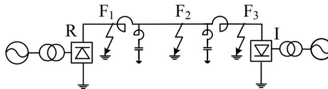
Fig.1. Unipolar HVDC system
