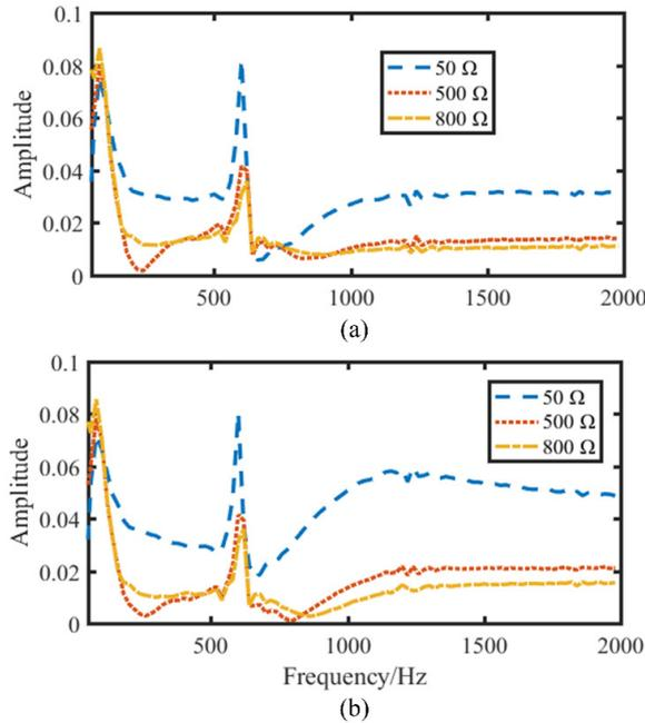
Fig.6. Amplitude frequency curves of different transition resistance (a)Location at Fd<sub>11</sub>; (b) Location at Fd<sub>22</sub>
