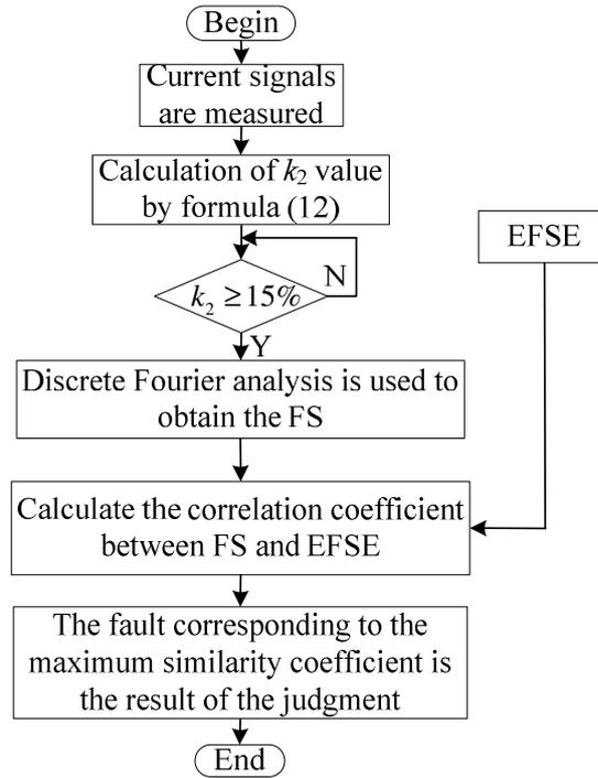
Fig.5. DC internal and external faults judging process
