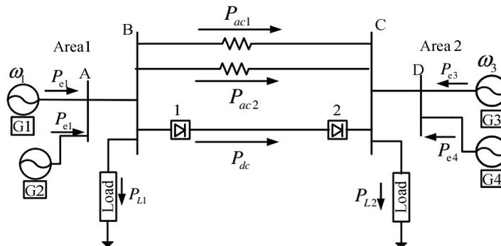
Fig.7. DC transmission system structure
