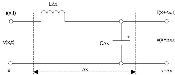
Figure 1. Approximate equivalent modelling of power distribution line.
