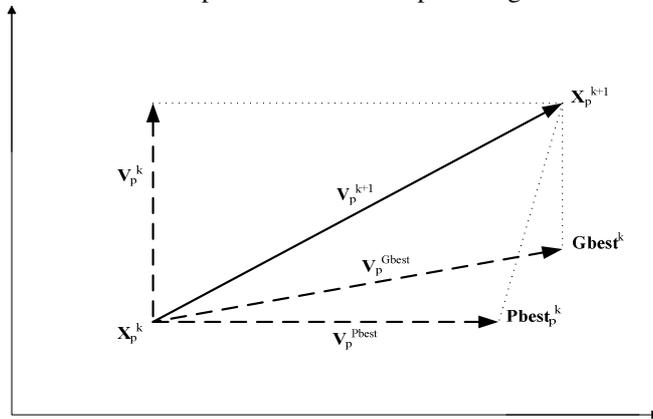
Figure 2. The PSO search mechanism of pth particle at kth iteration.
