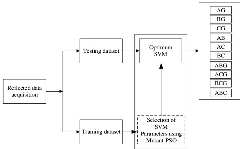
Figure 4. Proposed SVM using MPSO for fault classification.
