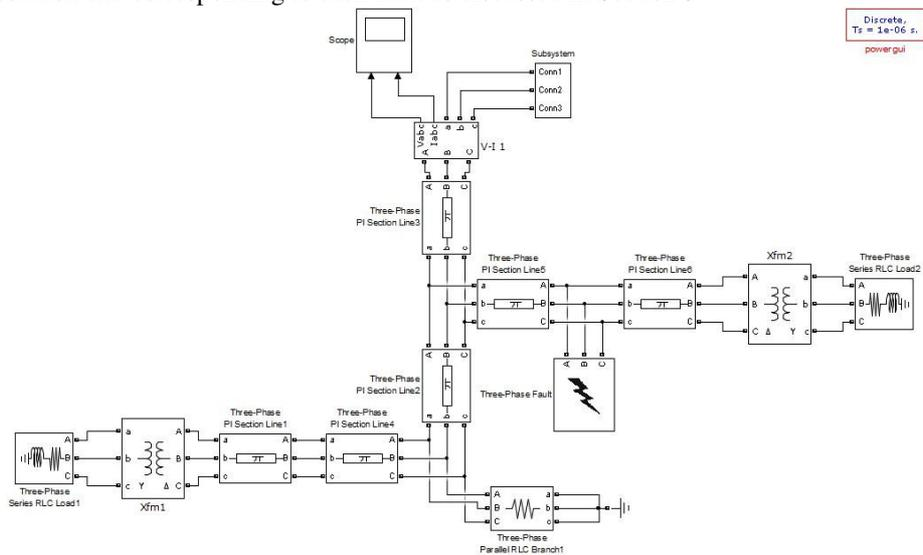
Figure 5. Simulating model of a two-branched distribution system.
