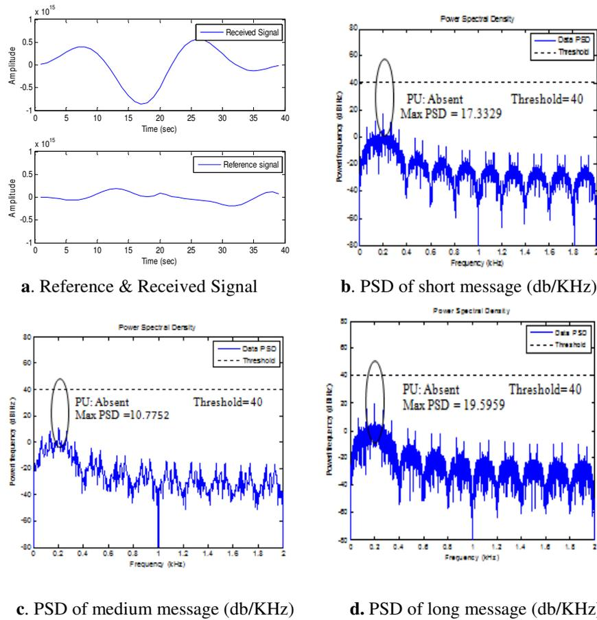
**Figure7: Reference/received signal and PSD plots for short, medium and long messages with set threshold =40db/KHz**
