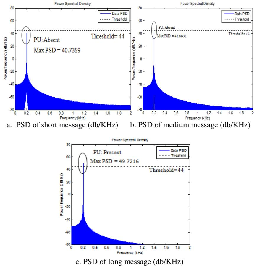
**Figure 5: PSD plots for short, medium and long messages with set threshold = 44db/KHz**
