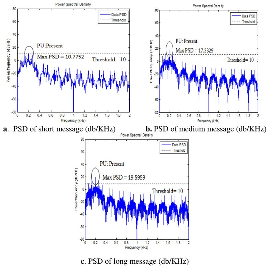
**Figure 9: Reference/received signal and PSD plots for short, medium and long messages with set threshold = 10db/KHz**
