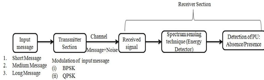
**Figure 1 : Block diagram to detect primary user using spectrum sensing**
