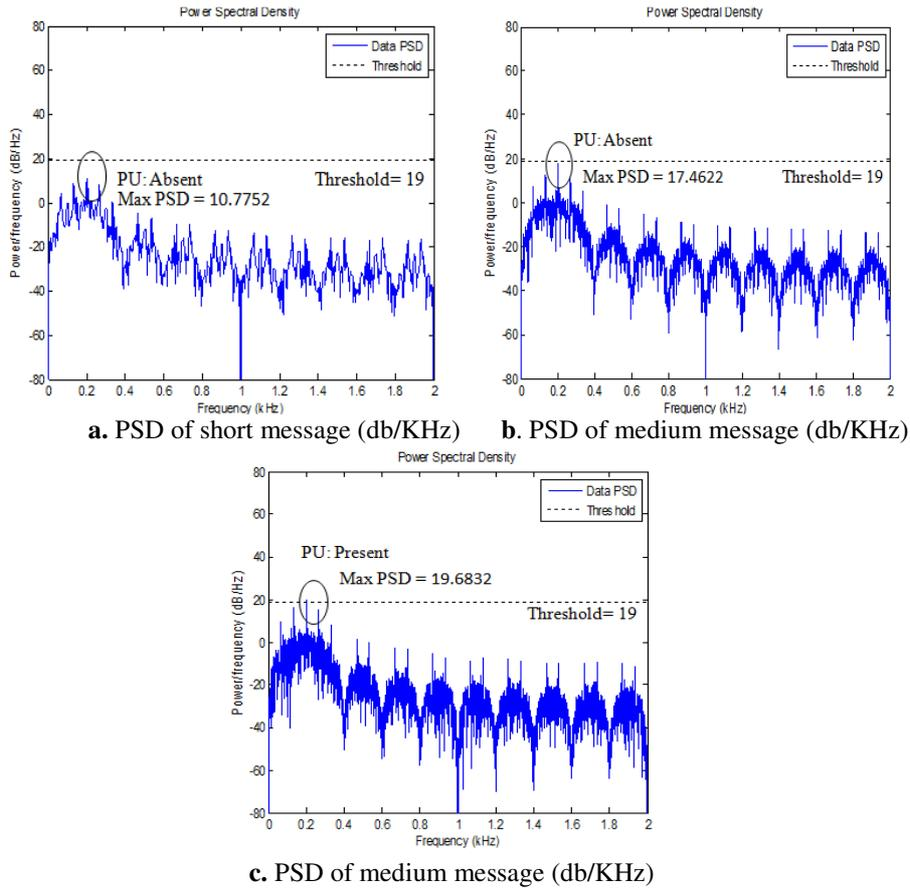
**Figure 8:** Reference/received signal and PSD plots for short, medium and long messages with set threshold = 19db/KHZ
