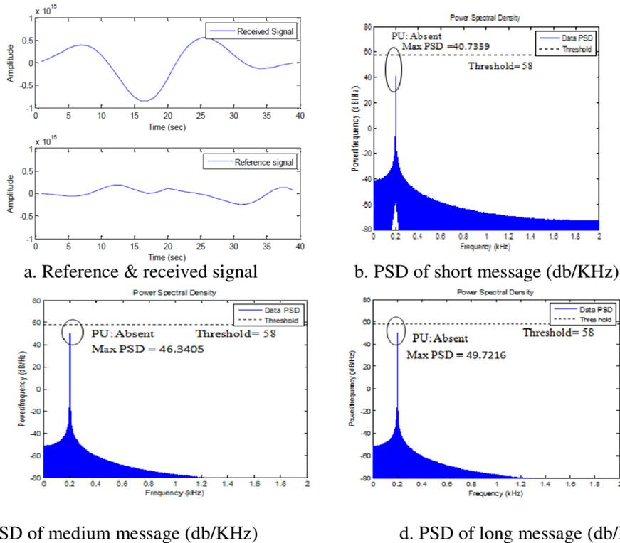
**Figure 4: Reference/received signal and PSD plots for short, medium and long messages with set threshold = 58db/KHz**
