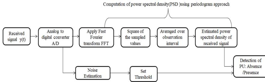
**Figure 2: Energy Detector based Spectrum Sensing**
