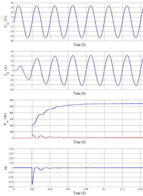
Fig.11. Waveforms of Input Parameters given To The Single Stage ZVS PFC Converter with voltage doubler unit
