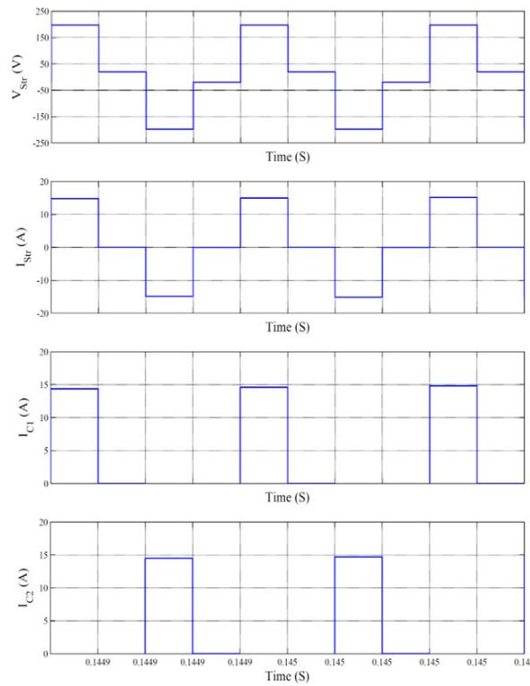
Fig.13. Internal waveforms of the voltage doubler
