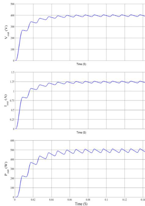
Fig.12. Waveforms Of The Obtained Specifications From The Single Stage ZVS PFC Converter with voltage doubler uni
