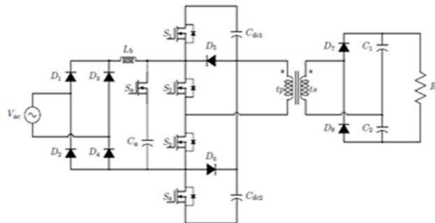
Fig.1: ZVS PFC Circuit With VD
