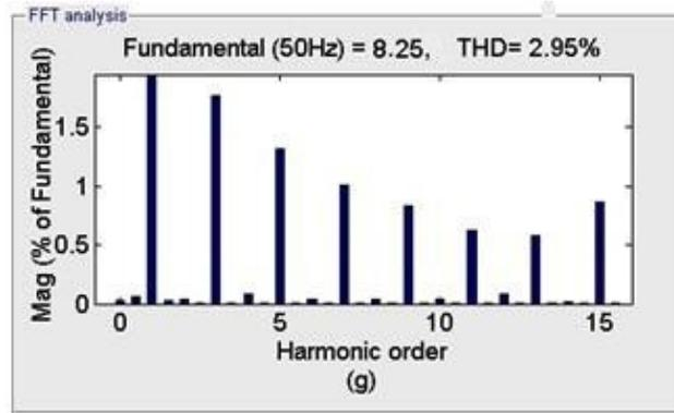
Fig.14. Harmonic spectra of the applied input current
