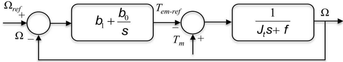
Fig. 7. Control structure of the turbine speed.
