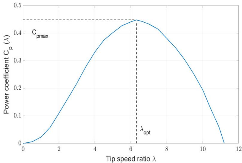
Fig. 3. Tidal stream turbine power coefficient curve.
