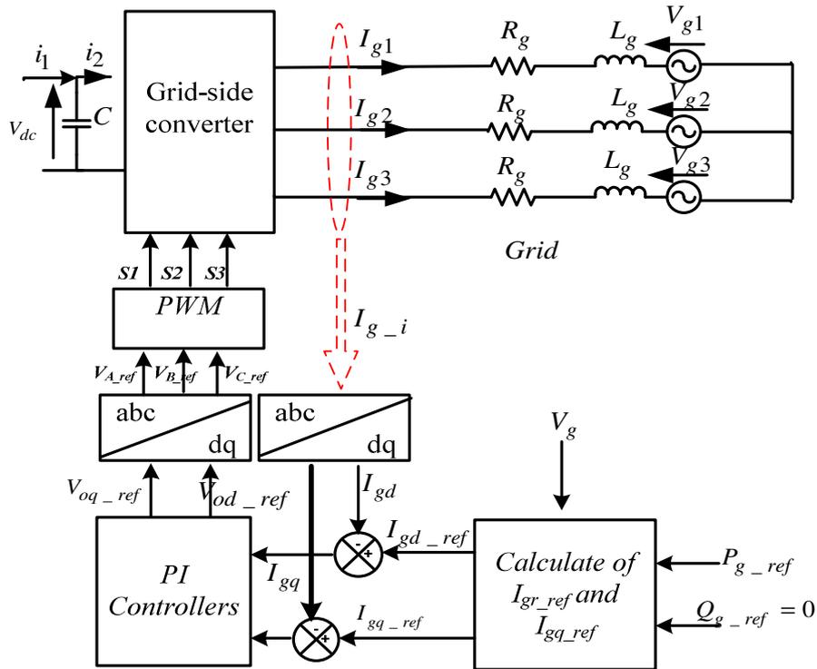
Fig. 9. Grid-side converter control.
