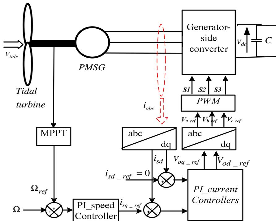
Fig. 6. Generator-side converter control.
