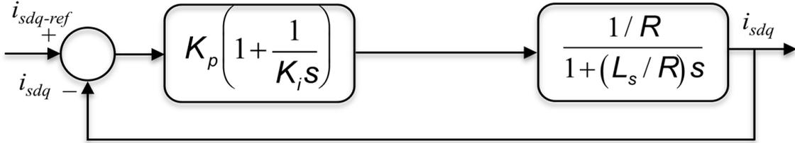
Fig. 8.  $i_{sdq}$  currents control structure.
