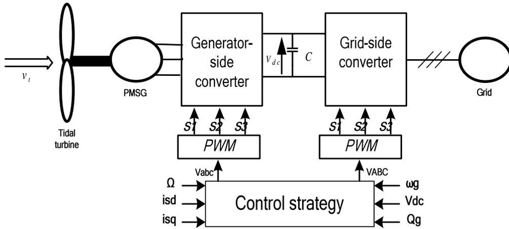
Fig. 2. Grid-connected PMSG-based tidal stream turbine system basic structure.
