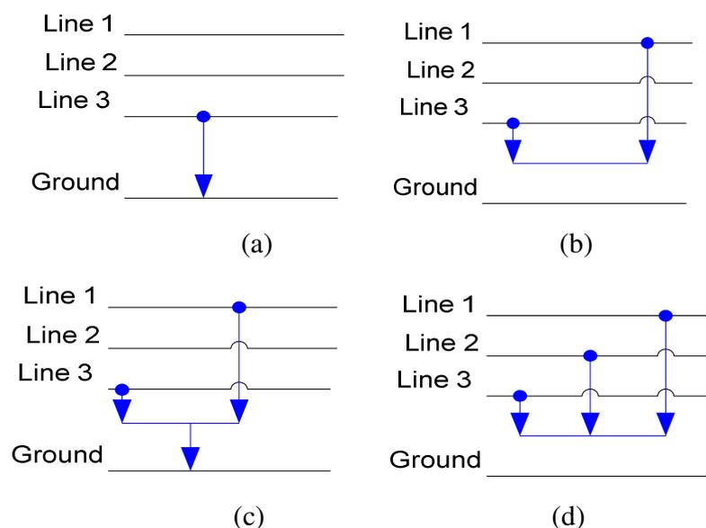
Fig. 1.(a) Single line-to-ground short-circuit fault, (b) Line-to-line short-circuit fault, (c) Line-to-line-to-ground short-circuit fault, (d) Three phases short-circuit fault.
