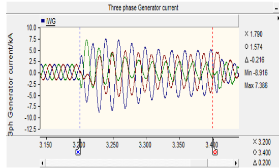
Fig.35 Three phase current of generator
