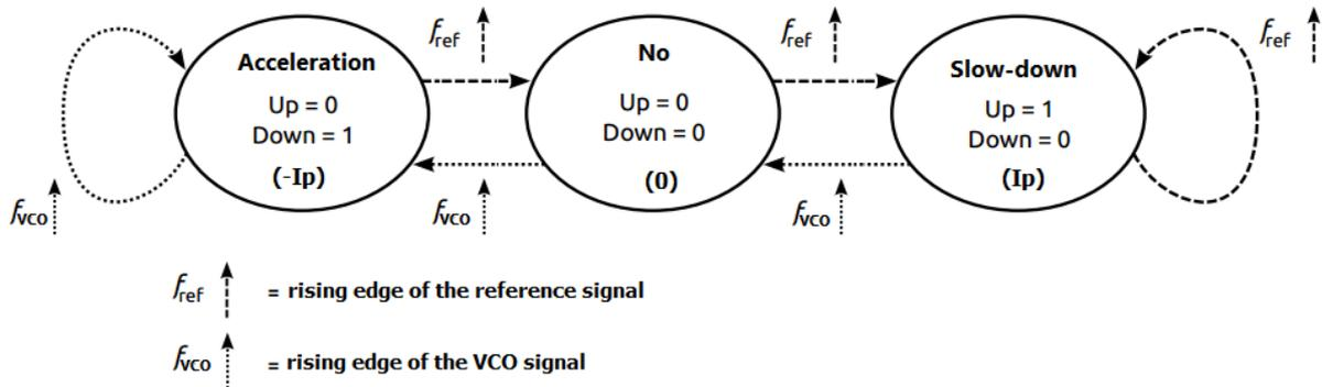
Fig.3. The operational states of the PFD
