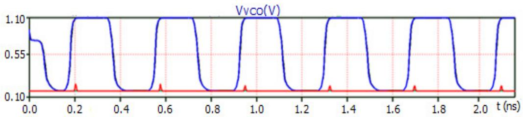
Fig.15. The VCO output at lock state,  $f_{\text{centre}}=3.70\text{GHz}$
