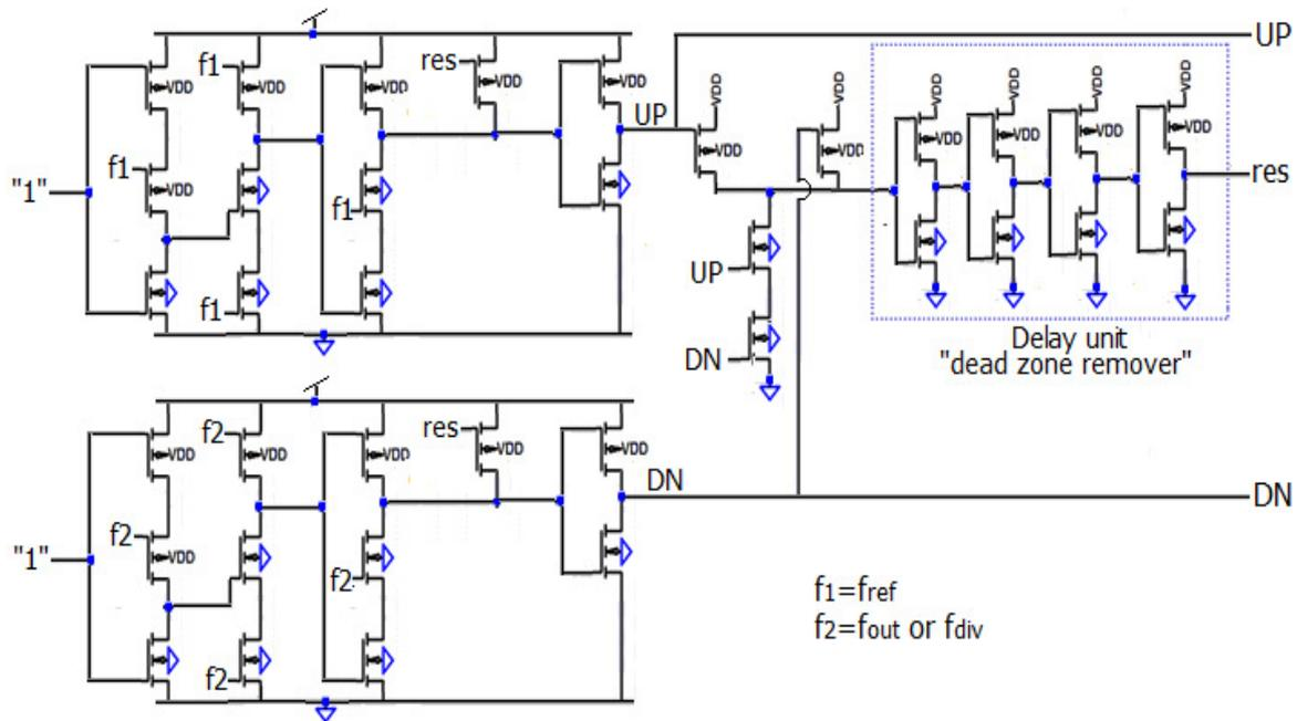
Fig.9. The PFD circuit diagram
