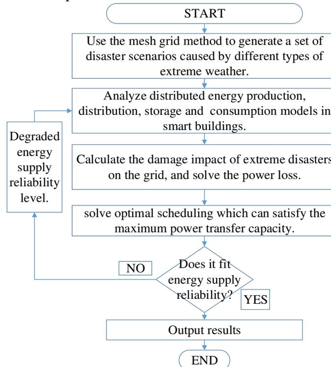
Figure 4 Flowchart of optimal dispatch of energy delivery after natural disasters
