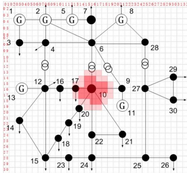
Figure 3 Network grid method to simulate the damage of IEEE 30-node system caused by natural disasters
