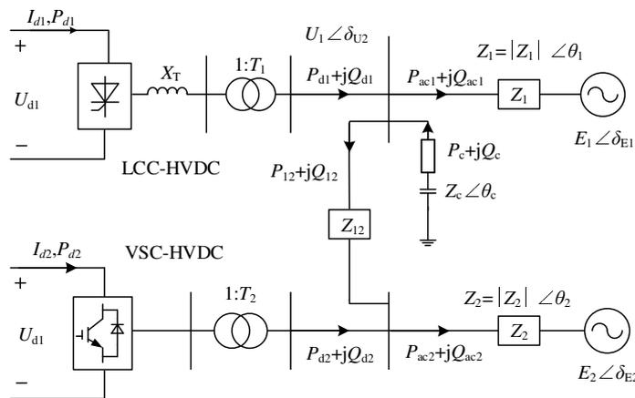
Figure 2. The HMIDC System
