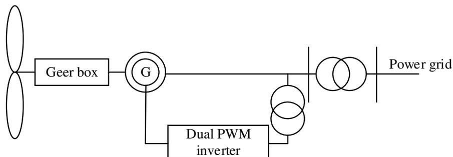
Figure 1. The DFIG-based WT model
