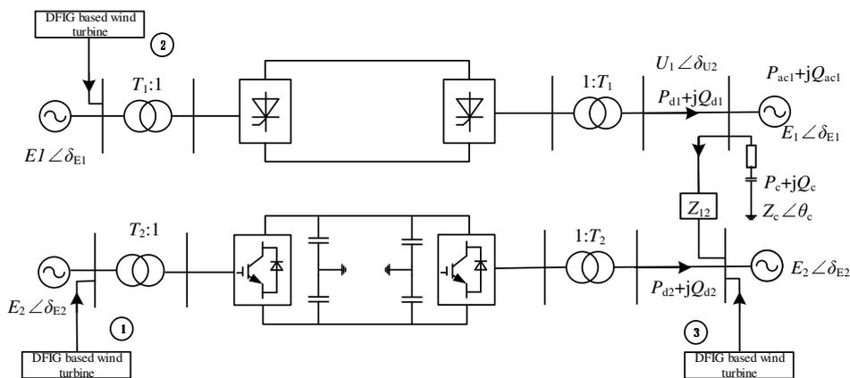
Figure 3. The HMIDC and DFIG-based WT connected to the Grid
