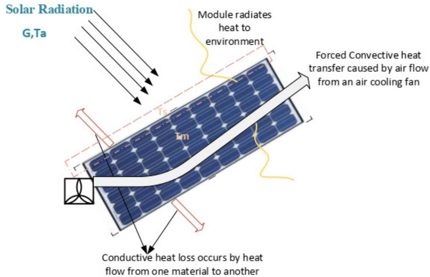
Fig. 5. Heat transfer schema with an air-cooling system of PV module.
