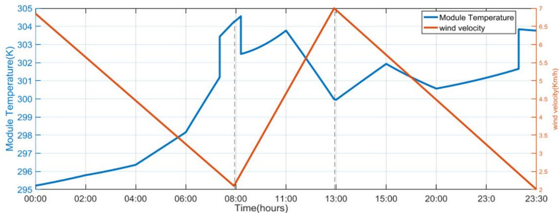
Fig. 10. Module temperature evolution as a function of air-cooling wind velocity
