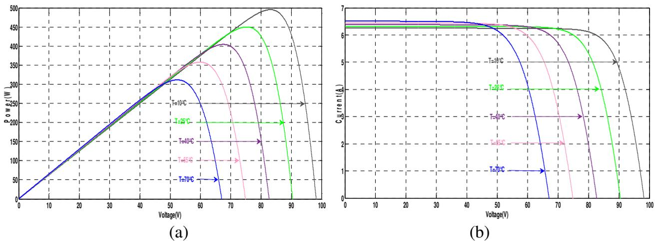
Fig. 2. (a) - I (V) Characteristic of a PV module for different temperatures
