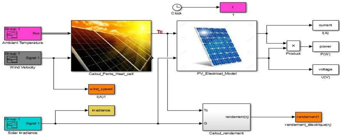
Fig. 8. Complete electrical-thermal model for improving PV performance
