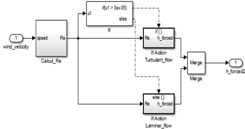
Fig. 6. Forced heat transfer coefficient calculation
