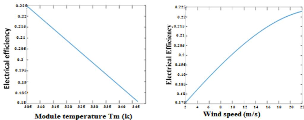
Fig. 12. Electrical efficiency as a function of Module temperature and wind velocity
