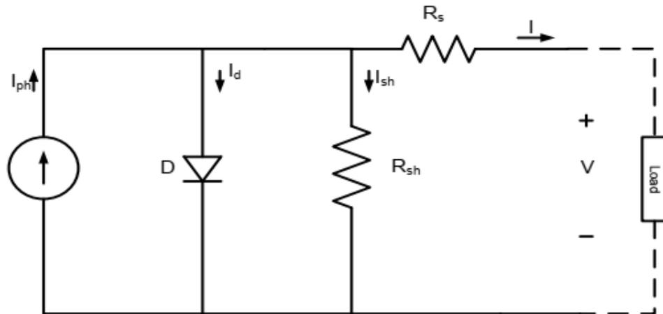
Fig. 1. Equivalent circuit of PV cell
