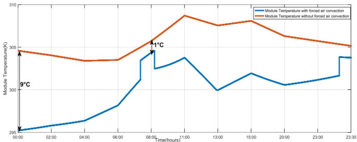
Fig. 11. Module temperature with and without air forced convection
