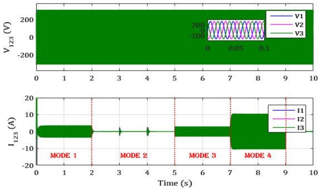
Fig. 7. (b). evolution of three phase voltage and current in grid in different operating modes
