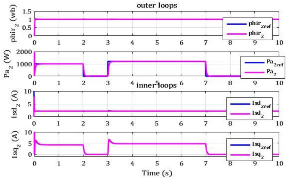
Fig. 8. (b). Second induction motor dynamic response using P-FOC
