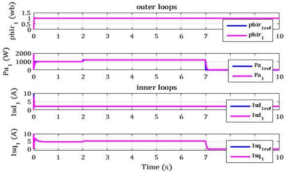
Fig. 8. (a). First induction machine performance using P-FOC
