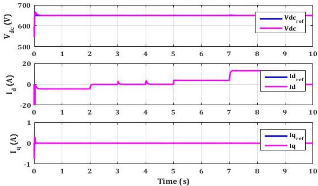
Fig. 7. (a). Grid connected PV system output response using VOC
