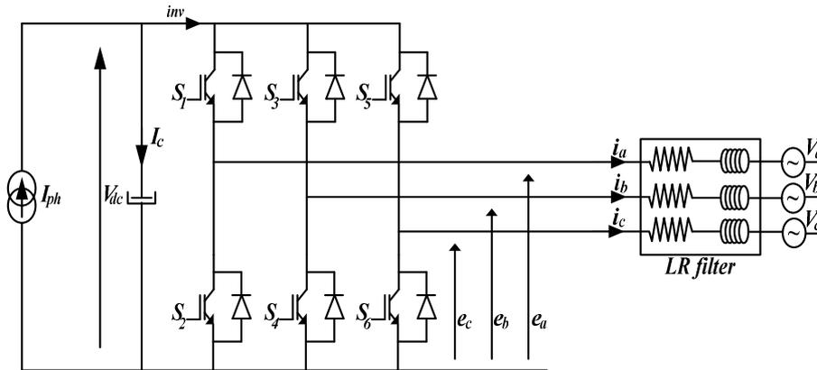
Fig. 4. Distribution network associated to VSI model
