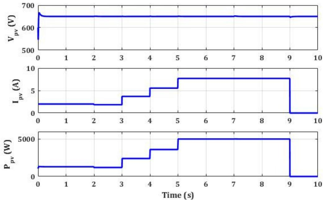
Fig. 6. Current, voltage and power in DC bus
