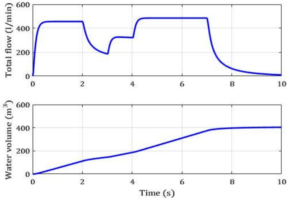
Fig. 11. Total flow and its corresponding pumped water volume
