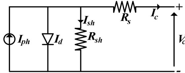
Fig. 3. Theoretical single diode photovoltaic module including shunt and series resistance
