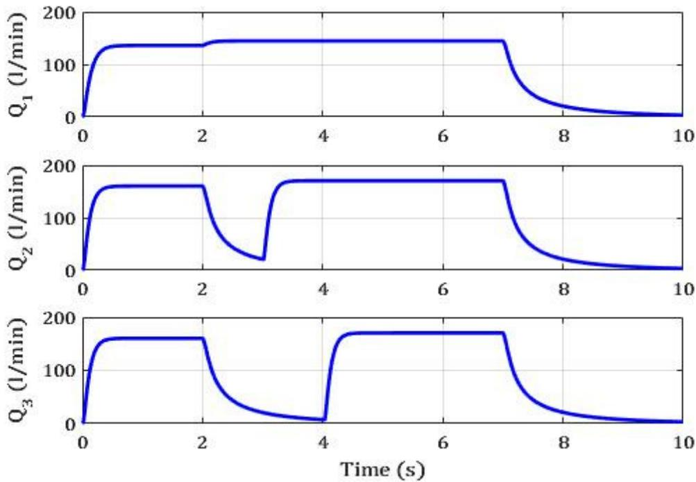
Fig. 10. (a). flow of water in three pumping system
