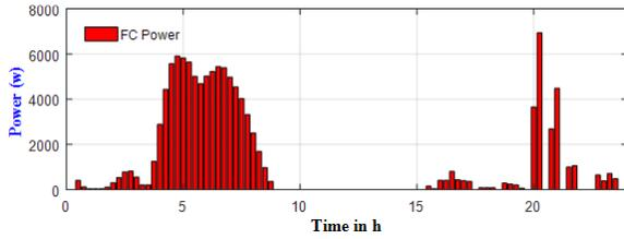
Figure 6. Optimal power product from Fuel Cell unit under scheduling policy 1
