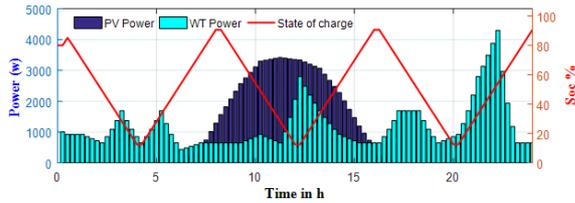
Figure 15. Optimal power RESs delivery in islanded mode under scheduling policy 3
