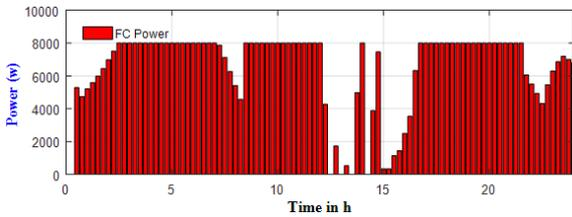
Figure 11. Optimal power product from Fuel Cell unit under scheduling policy 2
