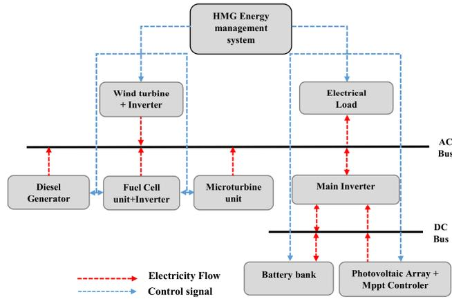
Figure 1. Hybrid AC/DC microgrid architecture
