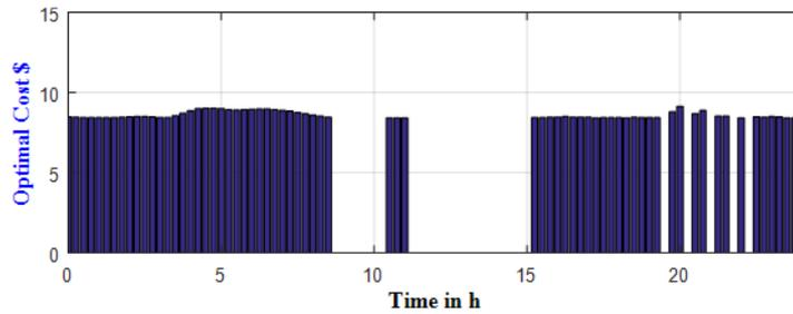
Figure 8. Optimal cost of using the CESs for each time interval under scheduling policy 1
