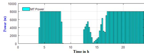
Figure 18. Optimal power product from Microturbine unit under scheduling policy 3
