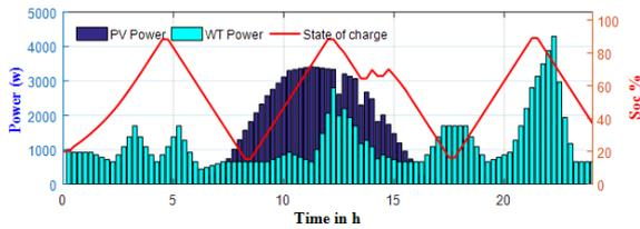
Figure 9. Optimal power RESs delivery in islanded mode under scheduling policy 2
