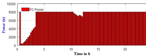
Figure 17. Optimal power product from Fuel Cell unit under scheduling policy 3
