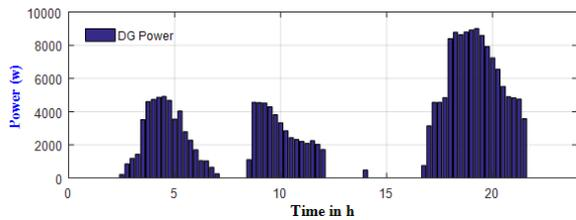
Figure 10. Optimal power product from Diesel Generator unit under scheduling policy 2
