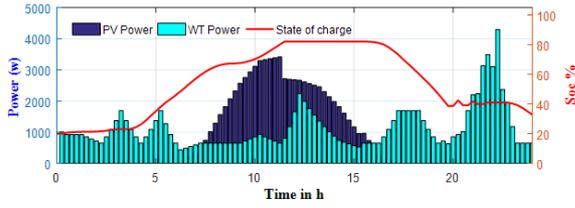
Figure 4. Optimal power RESs delivery in islanded mode under scheduling policy 1
