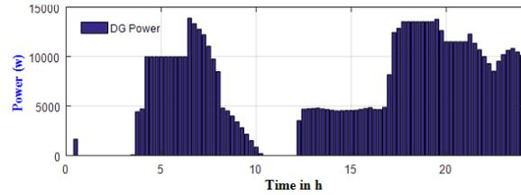
Figure 16. Optimal power product from Diesel Generator unit under scheduling policy 3
