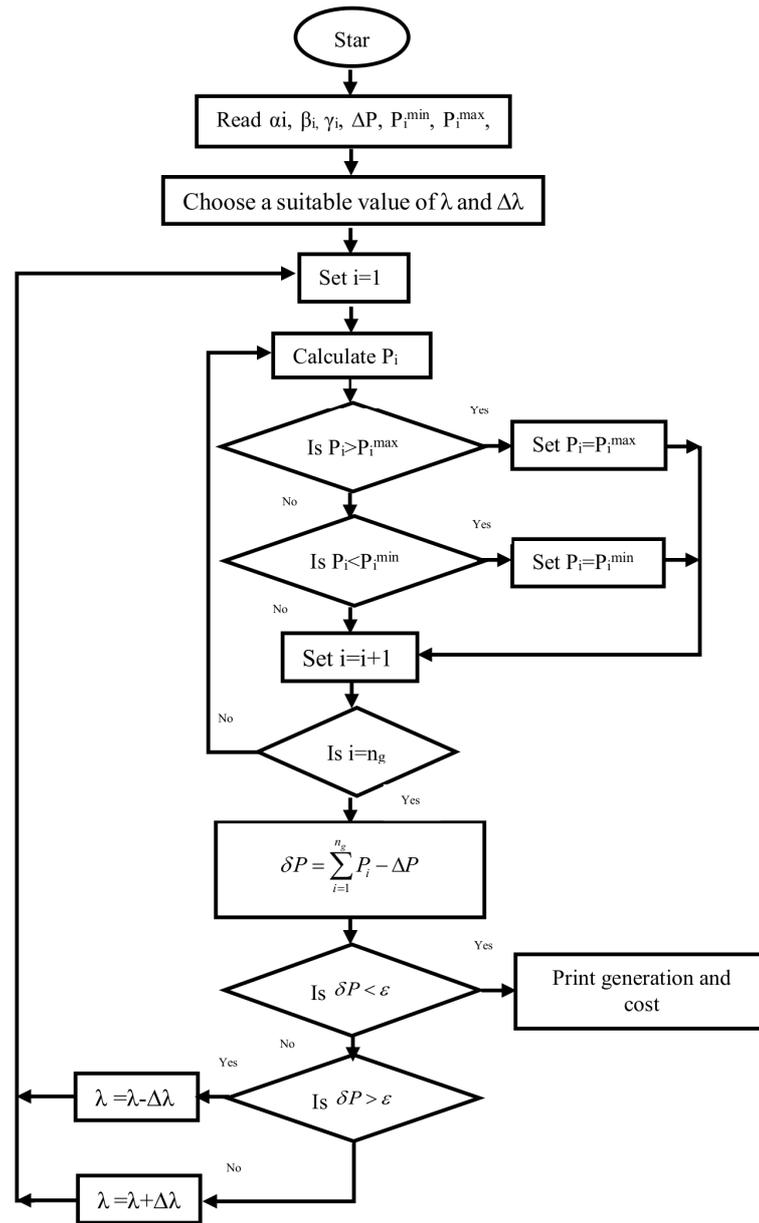
Figure 3. Flowchart of lambda iteration method for ELD
