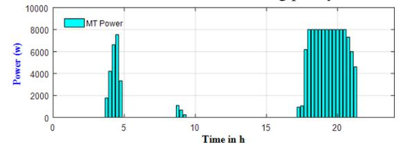
Figure 12. Optimal power product from Microturbine unit under scheduling policy 2
