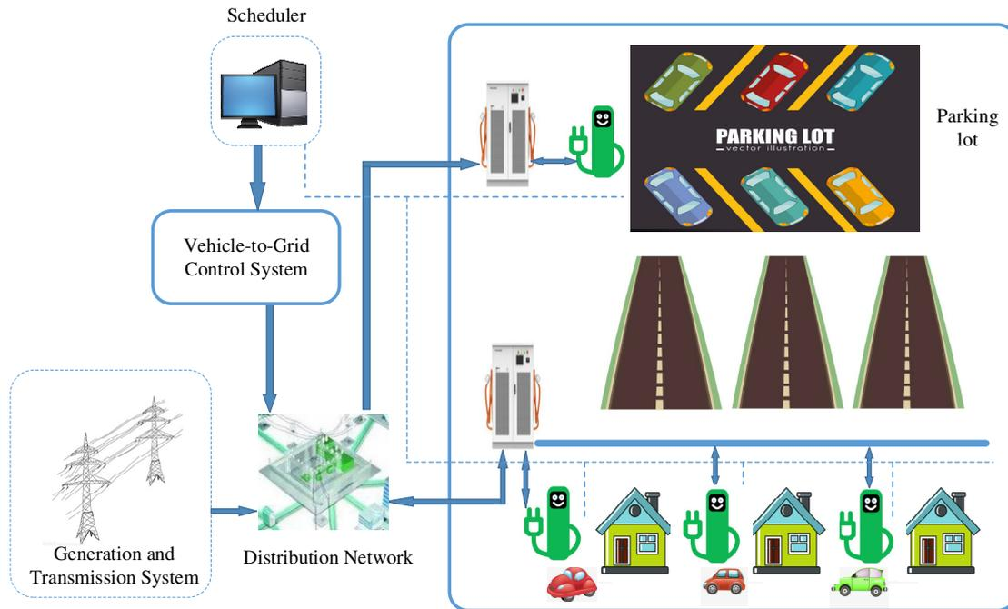
Figure 1: Configuration of a distribution system with EV PL
