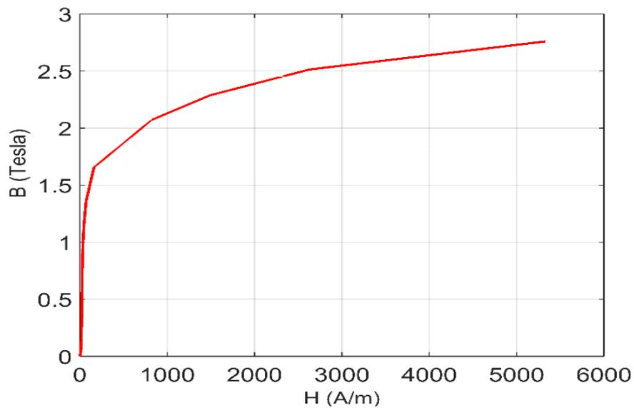
Fig. 3. B-H curve of the transformer
