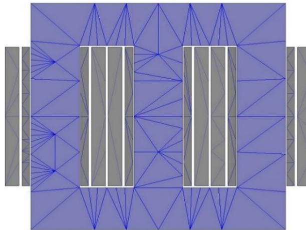
Fig. 9. 2-D. Mesh operation of Studied Transformer
