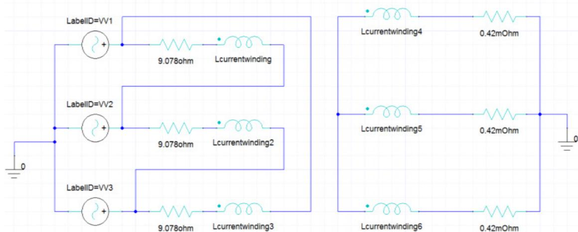
Fig. 7. External Excitation Circuit of Three-phase Transformer.
