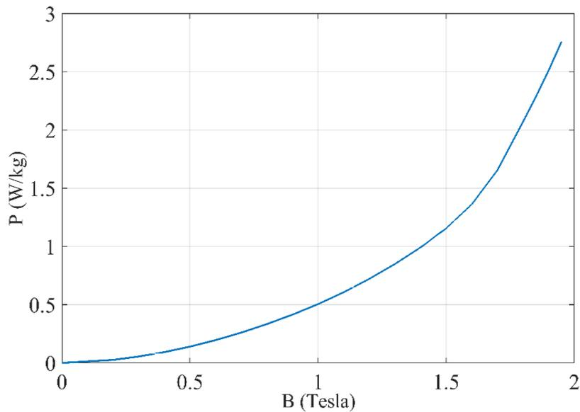
Fig. 4. B-P curve of the transformer
