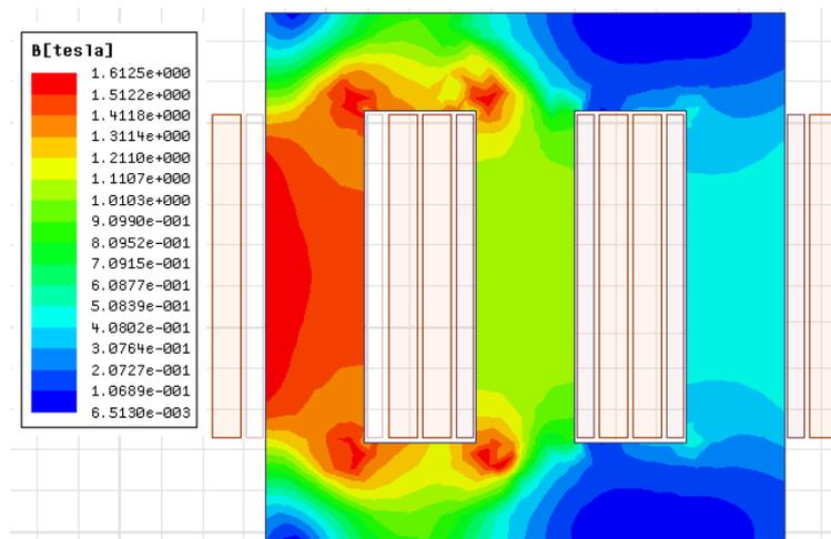
Fig. 11. 2-D. Magnetic flux density distribution
