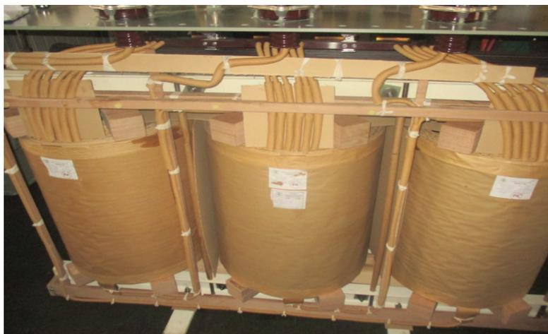
Fig. 1. Active parts of the transformer
