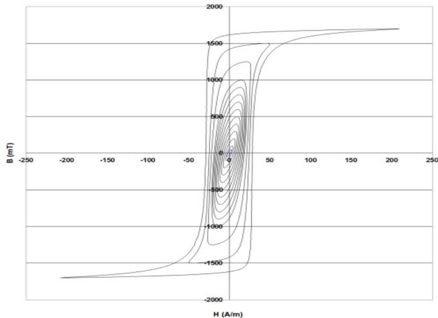
Fig. 5. Magnetization Curves of the core material
