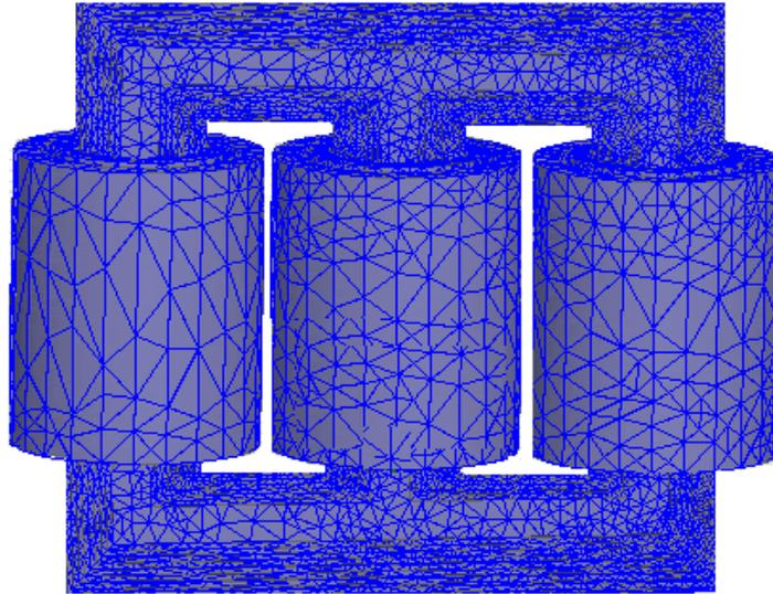
Fig. 8. 3-D. Mesh operation of Studied Transformer
