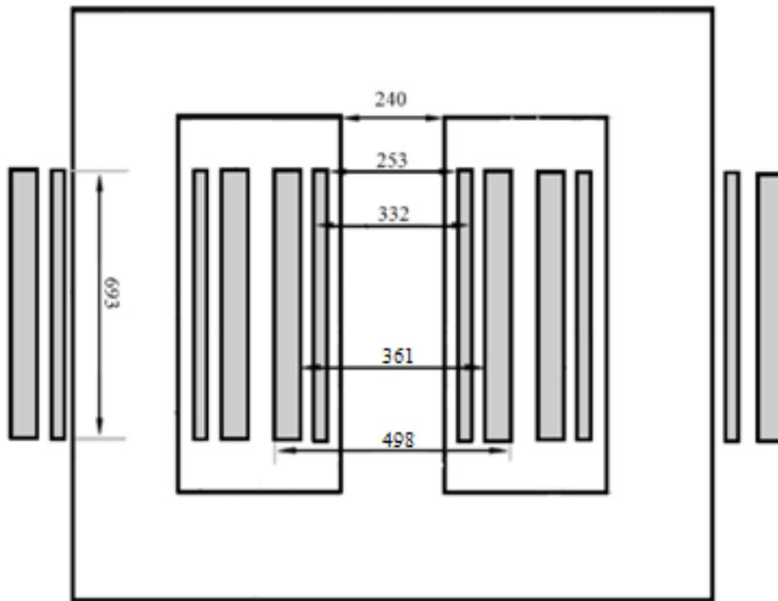
Fig. 2. 2-D geometry details of analyzed transformer (all dimensions are in mm)
