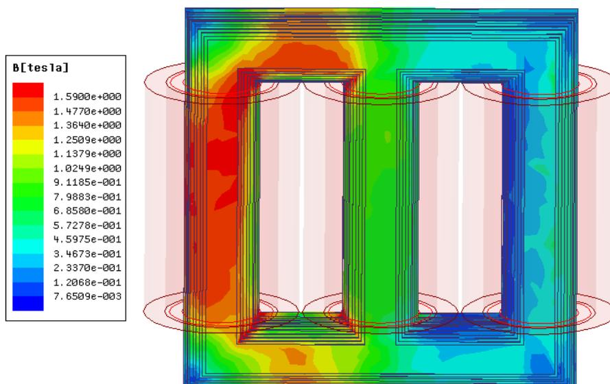
Fig. 10. 3-D. Magnetic flux density distribution
