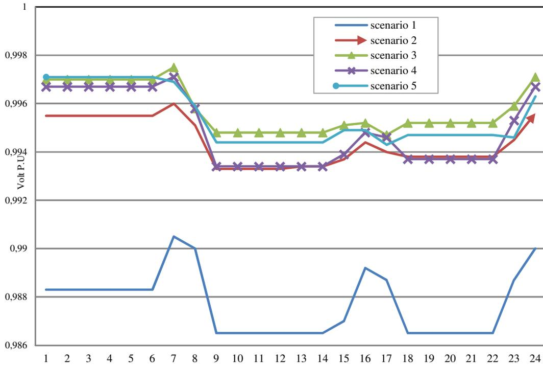
Fig.8. Lowest Voltage Magnitude of Cairo-59 bus RDN according to daily loading
