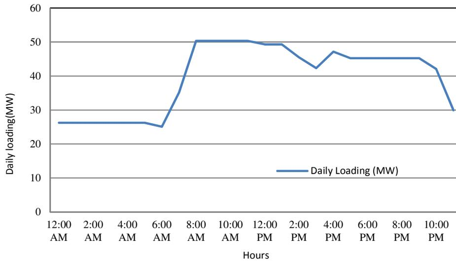
Fig.2. Daily loading profile of substation on bus 1
