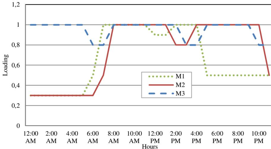
Fig.1. Daily loading curves M1, M2, and M3 for different busses in Cairo-59 bus RDN
