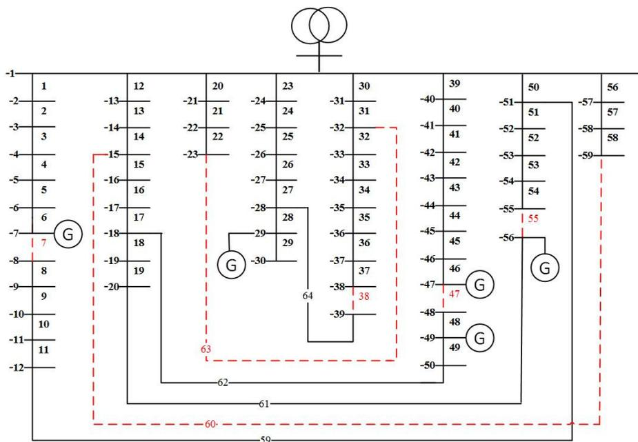
Fig.4. Cairo-59 bus system after reconfiguration and DG penetration
