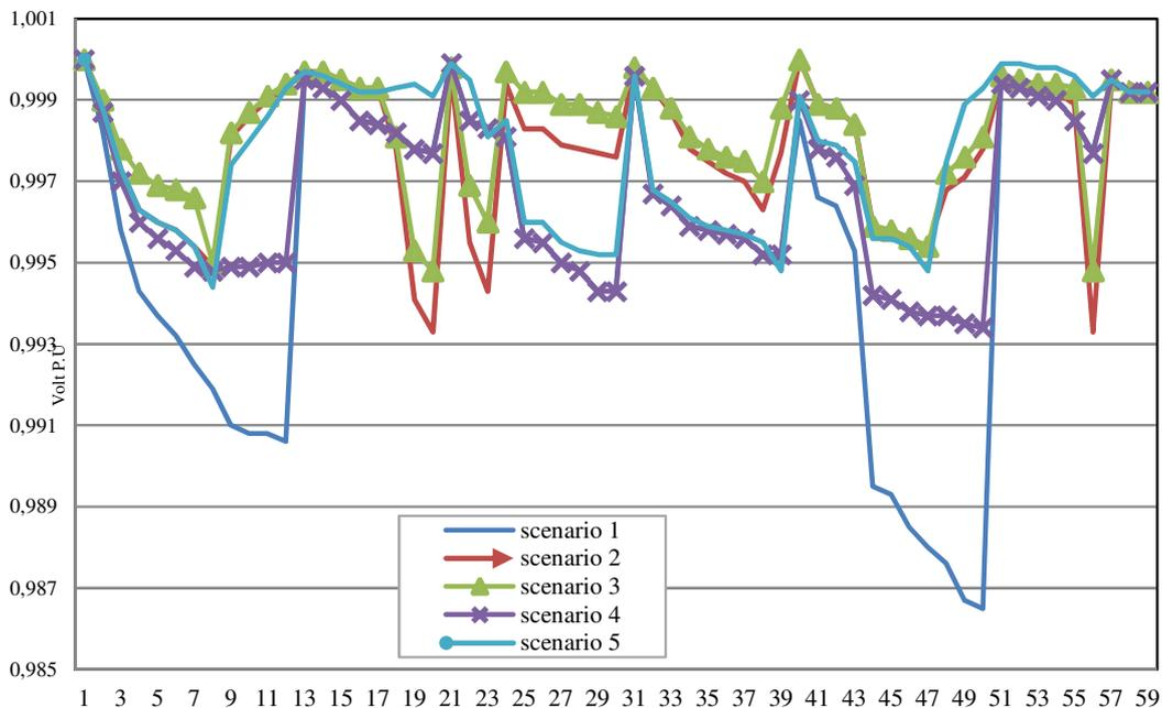
Fig.6. Voltage Profile of Cairo-59 bus Radial Distribution Network
