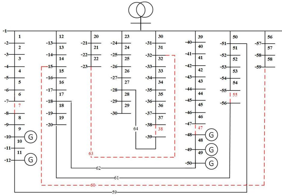
Fig.5. Cairo-59 bus system with DG penetration and after reconfiguration
