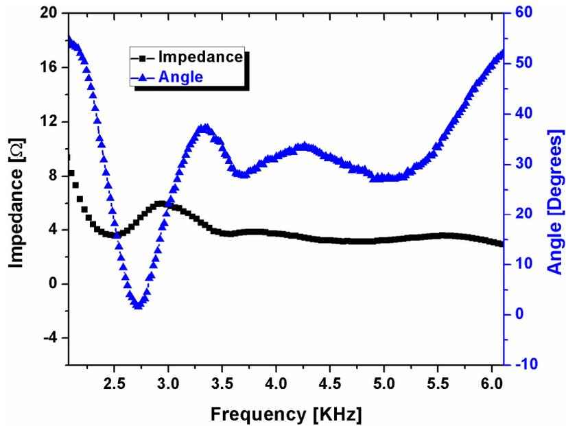
Fig.7. Impedance Results of Transducer with Matching Transformer Vs Frequency
