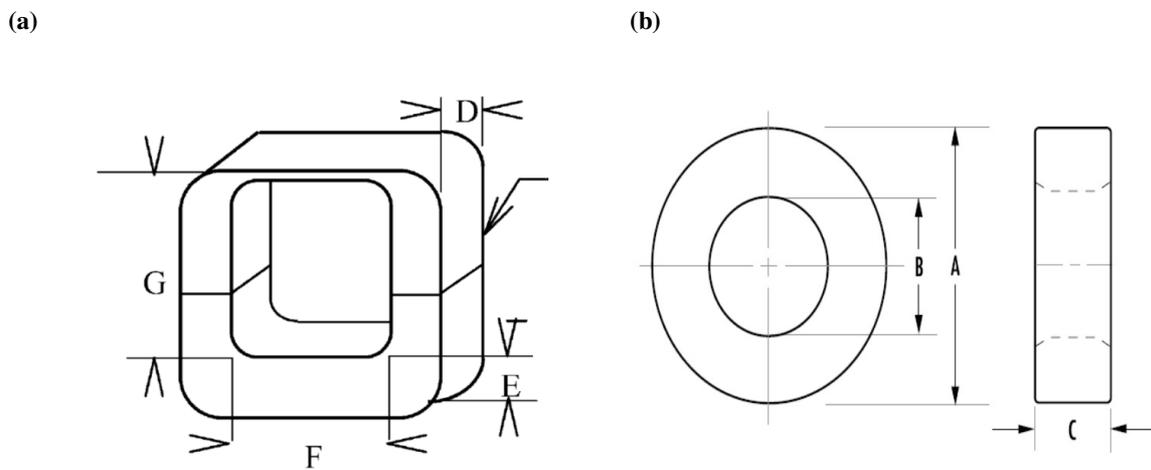
Fig.5. Schematic description of cores (a) C Type (b) Toroid Type
