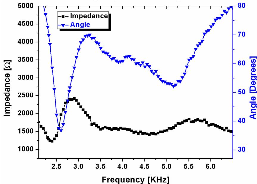
Fig.2. Impedance Results of Transducer Vs Frequency
