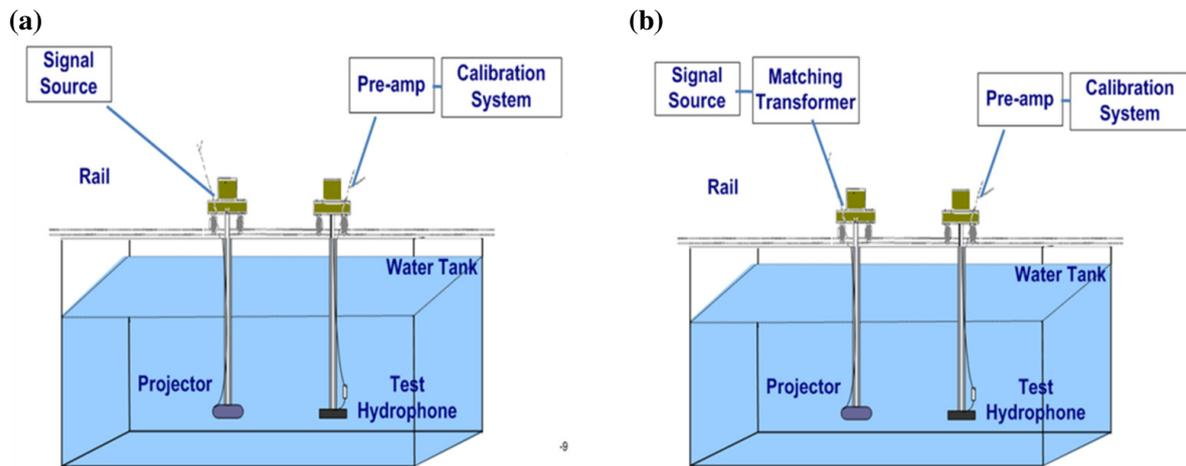
Fig.8. Schematic description of the source level measurement methodology of Transducer (a) without matching transformer and (b) with matching transformer
