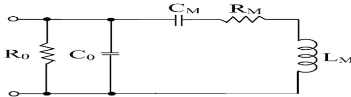
Fig.3. Lumped Equivalent Model of Transducer
