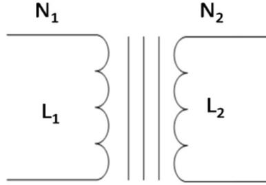
Fig.4. Schematic Description of Single Input/ Output based Ideal Transformer
