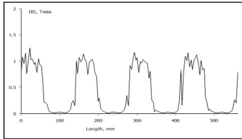
Fig. 11 - Machine simulation with rotor of salient poles from Fe-2%P sintered - Air-gap flux density.
