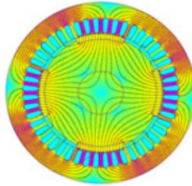
Fig.16 – Machine simulation with rotor of straight poles from Fe-2%P sintered - Flux lines in the longitudinal plane of the machine.
