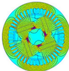
Fig. 18 - Machine simulation with rotor of embedded magnets from M15 steel sheet - Flux lines in the longitudinal plane of the machine.
