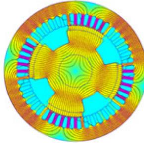
Fig. 12 - Machine simulation with rotor of salient poles from Fe-2%P sintered - Flux lines in the longitudinal plane of the machine.
