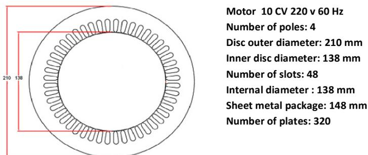
Fig. 5 – Schematic of machine stator sheets.
