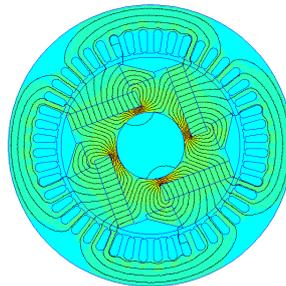
Fig. 20 - Machine simulation with rotor of embedded magnets from sintered Fe-2%P alloy - Flux lines in the longitudinal plane of the machine
