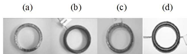
Fig. 3 Sample preparation steps: (a) isolating (b) secondary winding, (c) isolating and (d) the primary winding
