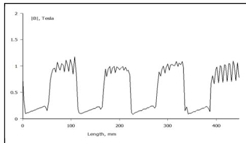
Fig.13 – Machine simulation with rotor of straight poles from M15 steel sheet - Air-gap flux density.
