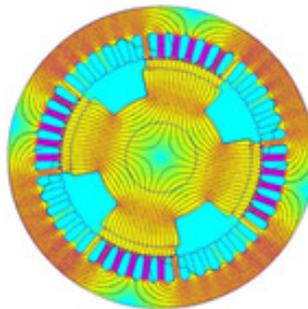
Fig. 10 - Machine simulation with rotor of salient poles from M15 steel sheet - Flux lines in the longitudinal plane of the machine.
