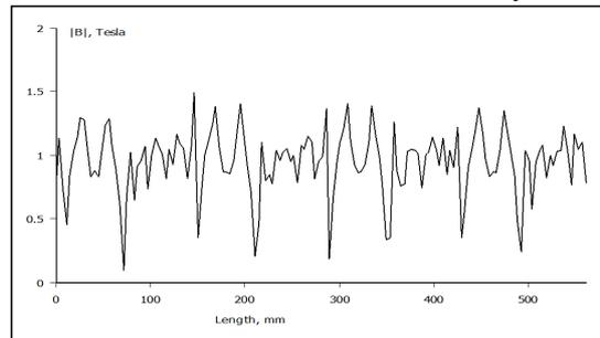
Fig. 9 - Machine simulation with rotor of salient poles from M15 steel sheet - Air-gap flux density.
