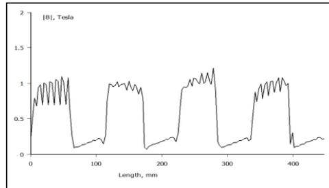
Fig.15 – Machine simulation with rotor of straight poles from Fe-2%P sintered - Air-gap flux density.
