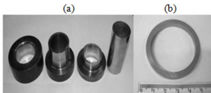
Fig.1 - Samples in the form of ring - (a) Die - (b) Specimen. (scale in centimeters).
