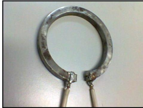
Fig.4 – Segmented ring for measuring electrical resistivity.
