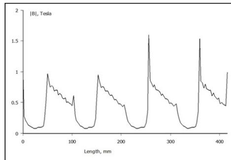
Fig. 17 - Machine simulation with rotor of embedded magnets from M15 steel sheet - Air-gap flux density.
