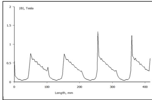
Fig. 19 – Machine simulation with rotor of embedded magnets from sintered Fe-2%P alloy - Air-gap flux density.
