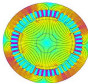
Fig.14 – Machine simulation with rotor of straight poles from M15 steel sheet - Flux lines in the longitudinal plane of the machine.
