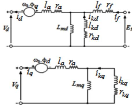
**Fig.3.** SPSG (a) d-axis equivalent circuit(b) q-axis equivalent circuit
