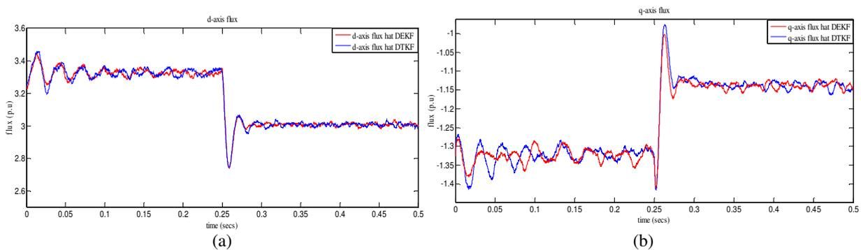
Fig.10. d-q axis estimated fluxes obtained from DTKF and DEKF (a) d-axis current (b) q-axis current.
