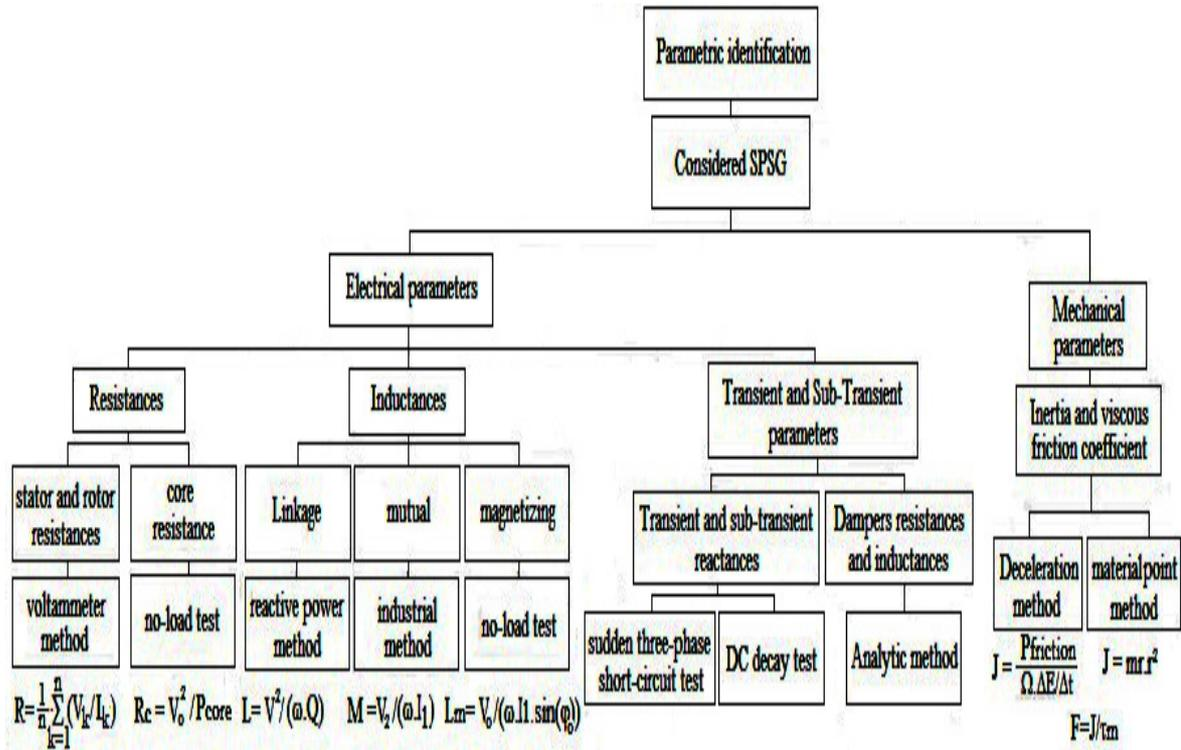
Fig.2. Off-line parameters identification method of considered SPSG.
