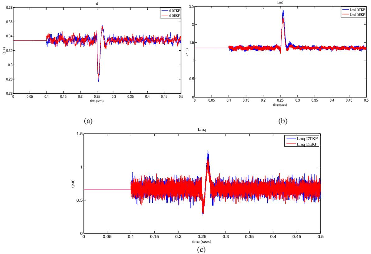
Fig.11. Estimated parameters of the steady state (a)  $r_f$  (b)  $L_{md}$  (c)  $L_{mq}$
