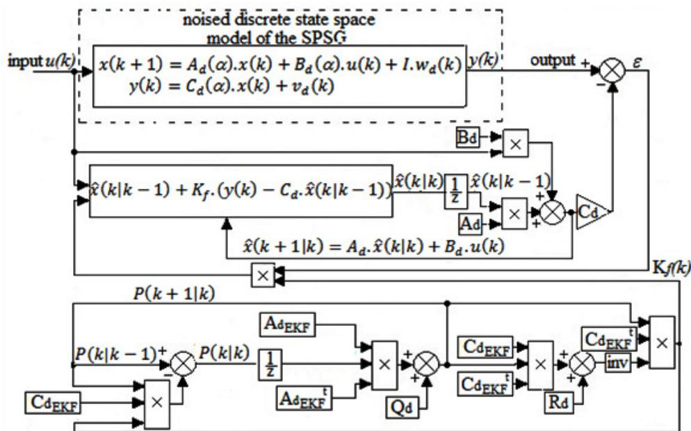
Fig.6. Chart of EKF principle
