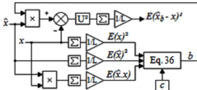
Fig.7. Principle of the proposed DBEKF
