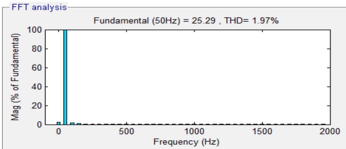
Fig 12: Total Harmonics distortion of source currents.
