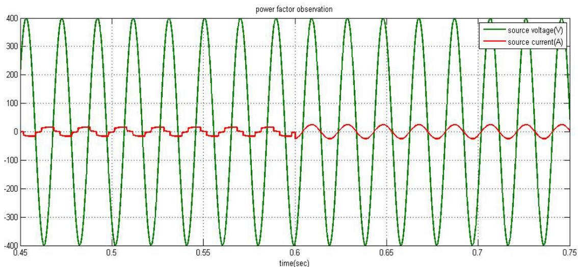
Fig 10: Power factor maintained unity when the Statcom is acting from 0.6 sec with  $I_{dq}$  controller.
