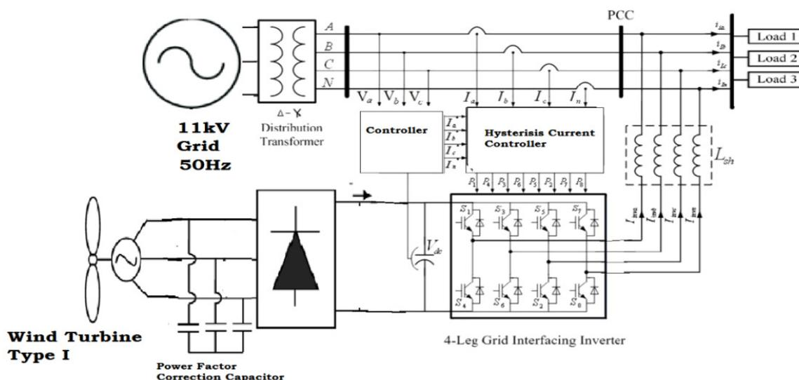
Fig.1. Block diagram of grid connected wind generation system at distribution level.
