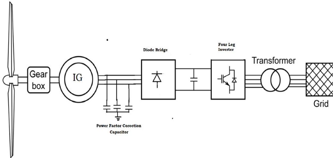
Fig. 2. Type I Wind Generation with DC Link equivalent diagram.
