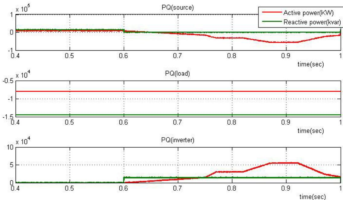
Fig 7: Simulated output wave forms of Source, load and Compensated active and re-active powers with Unit Vector controller.
