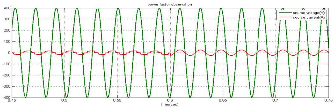
Fig 6: Power factor maintained unity when the inverter is connected from 0.6 sec with Unit Vector controller.
