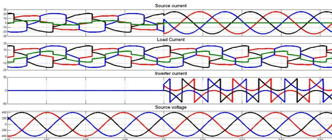
Fig 9: Three phase wave forms of source current, Load current, inverter currents and source voltage
