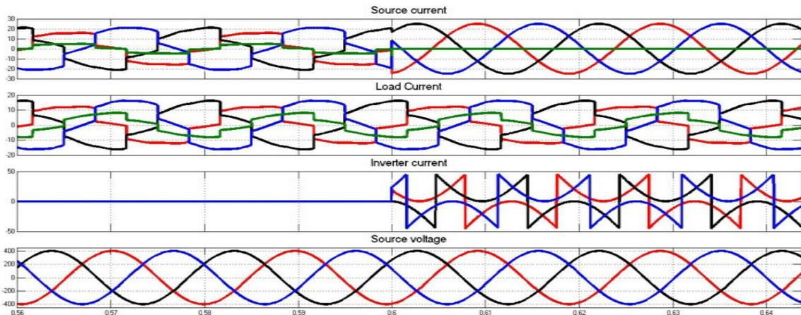
Fig 5: Three phase wave forms of source current, Load current, inverter currents and source voltage
