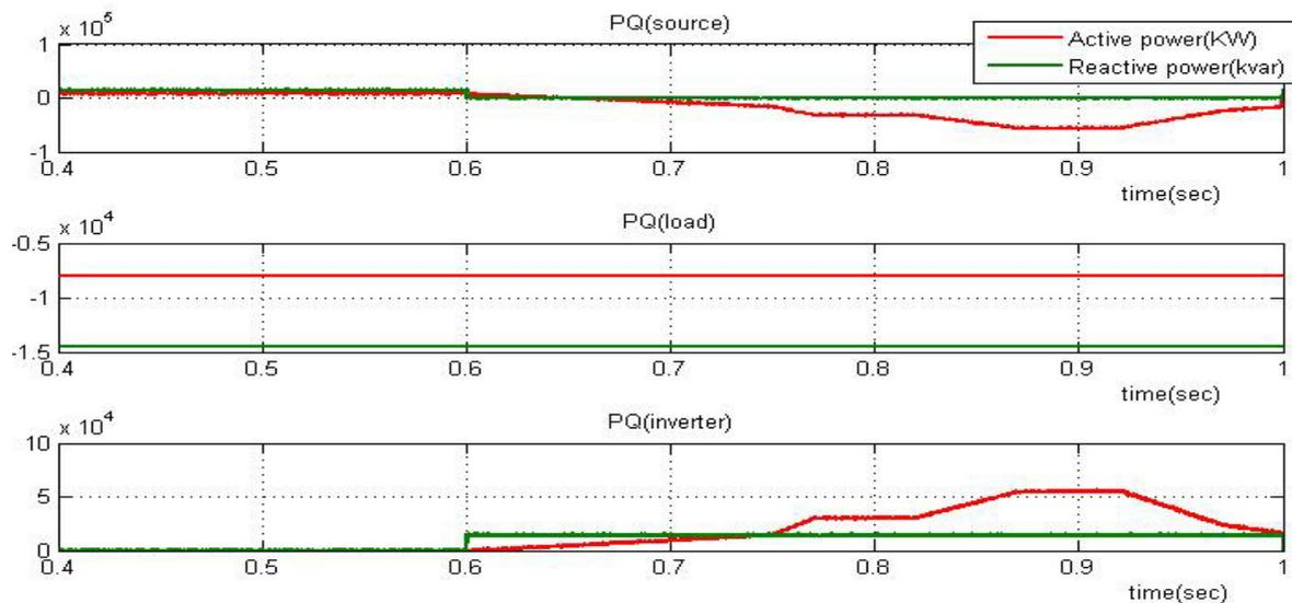
Fig 11: Simulated output wave forms of Source, load and Compensated active and re-active powers with  $I_{dq}$  controller.
