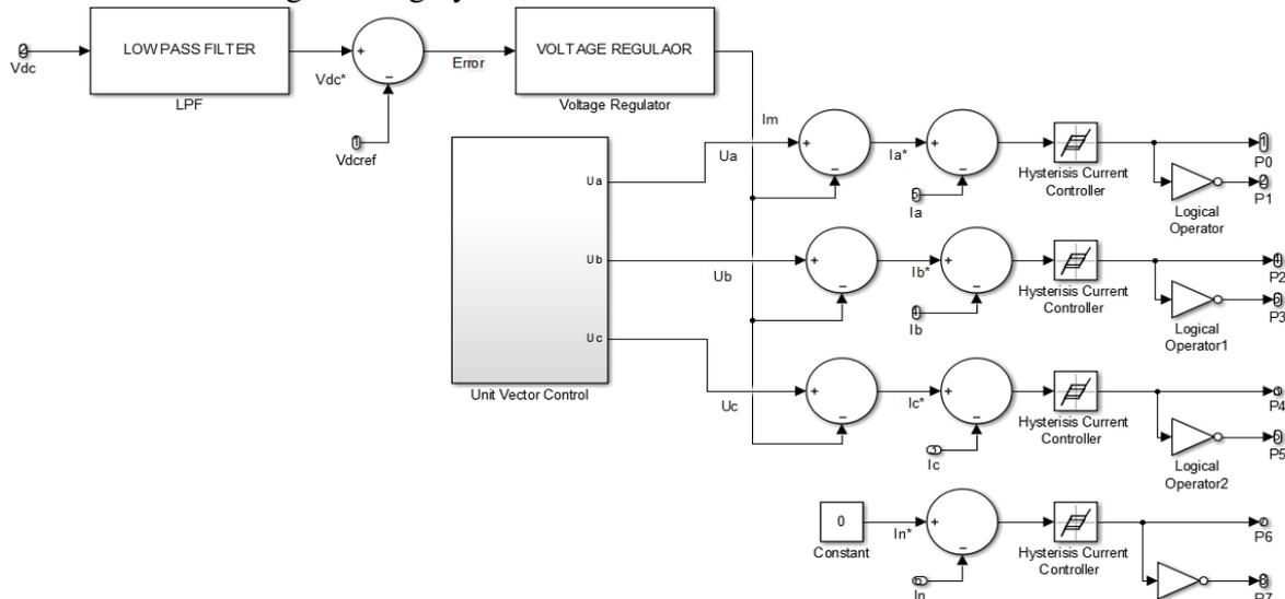
Fig.3 Block diagram representation of Unit vector control scheme
