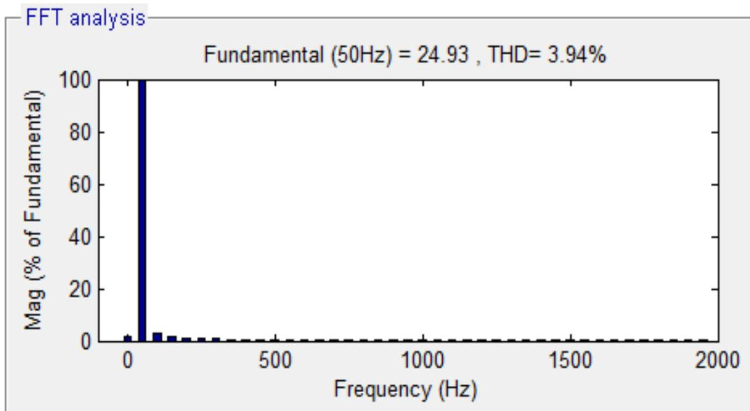
Fig 8: Total Harmonics distortion of source currents.
