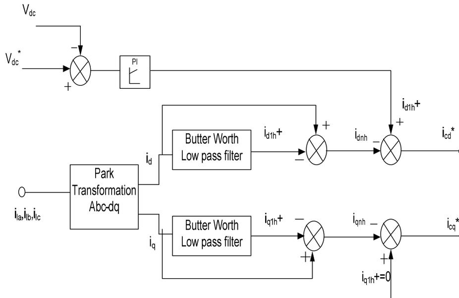
Fig.4. Transformation and injection of harmonic current.
