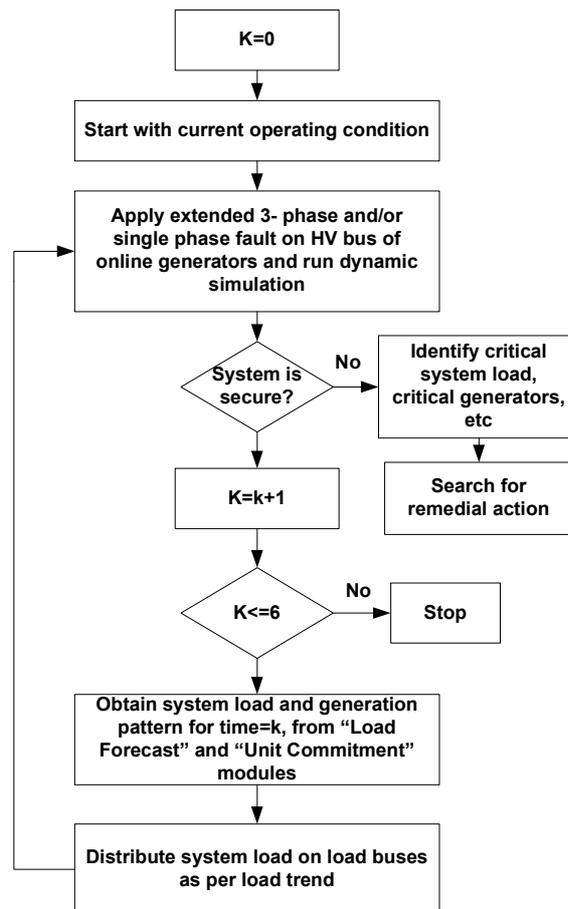
Fig.3: structure of early warning system based on dynamic security assessment
