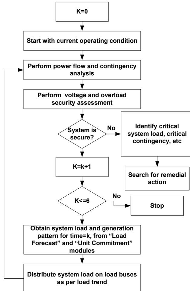
Fig.2: structure of early warning system based on steady state security assessment
