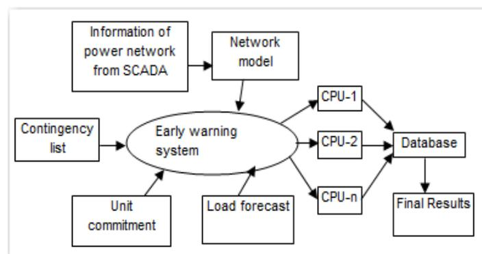
Fig.1: integration of proposed system with existing SCADA/ EMS applications
