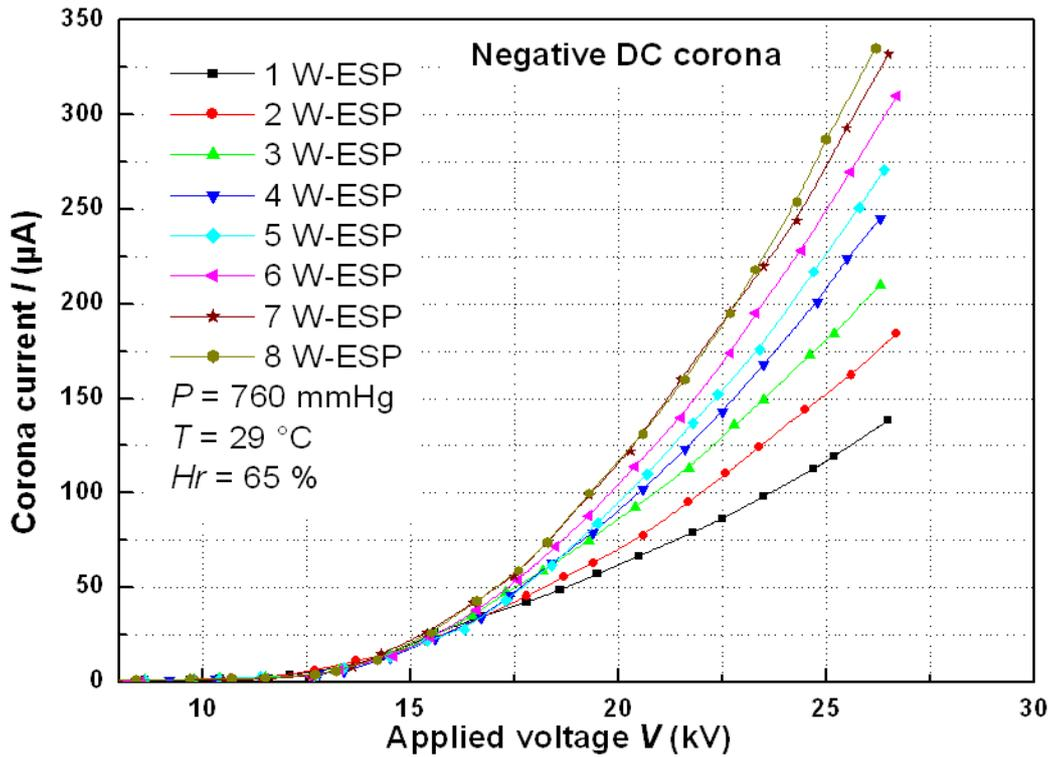
**Fig. 3.** Current-voltage characteristics for the DC negative corona.
