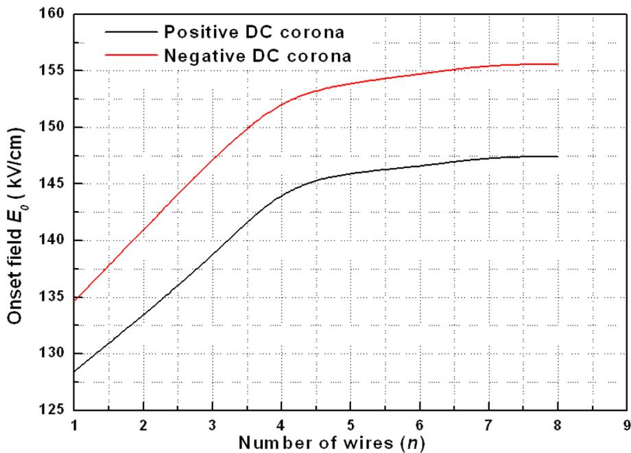
**Fig. 7.** Onset corona field versus of the wires number.
