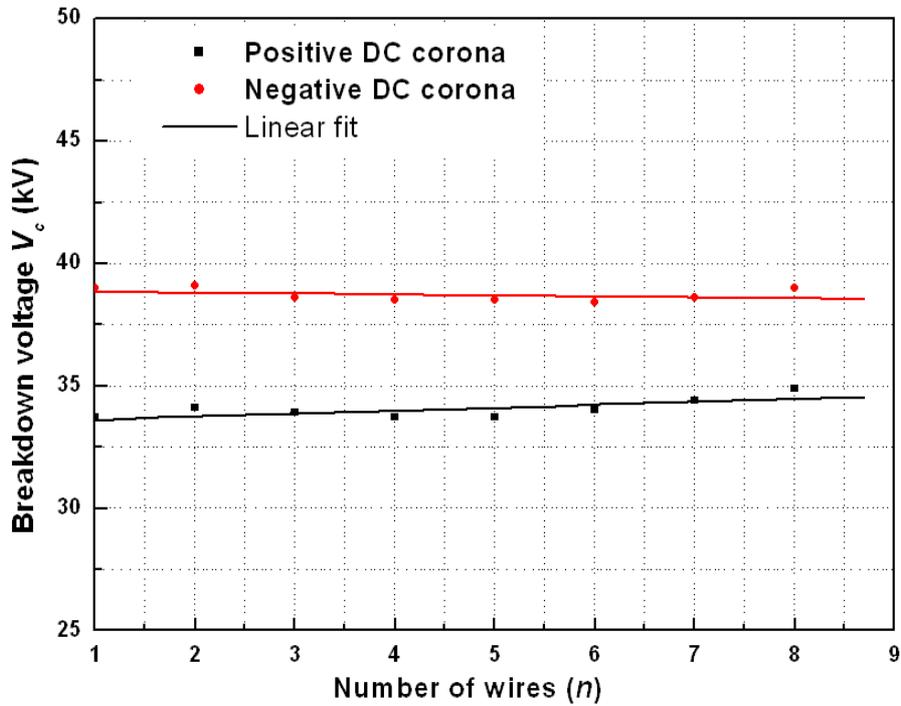
**Fig. 8.** Breakdown voltage versus the number of discharging wires.
