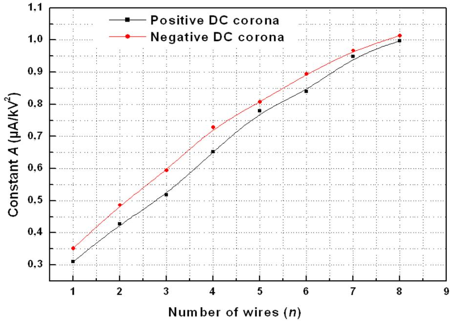
**Fig. 11.** Variation of the dimensional constant  $A$  with the number of wires.
