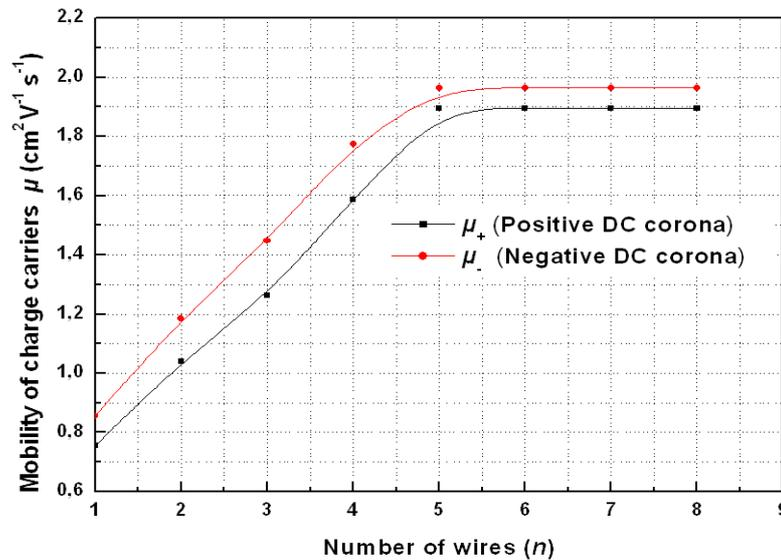
**Fig. 13.** The apparent mobility of the charge carriers by function of wires number.
