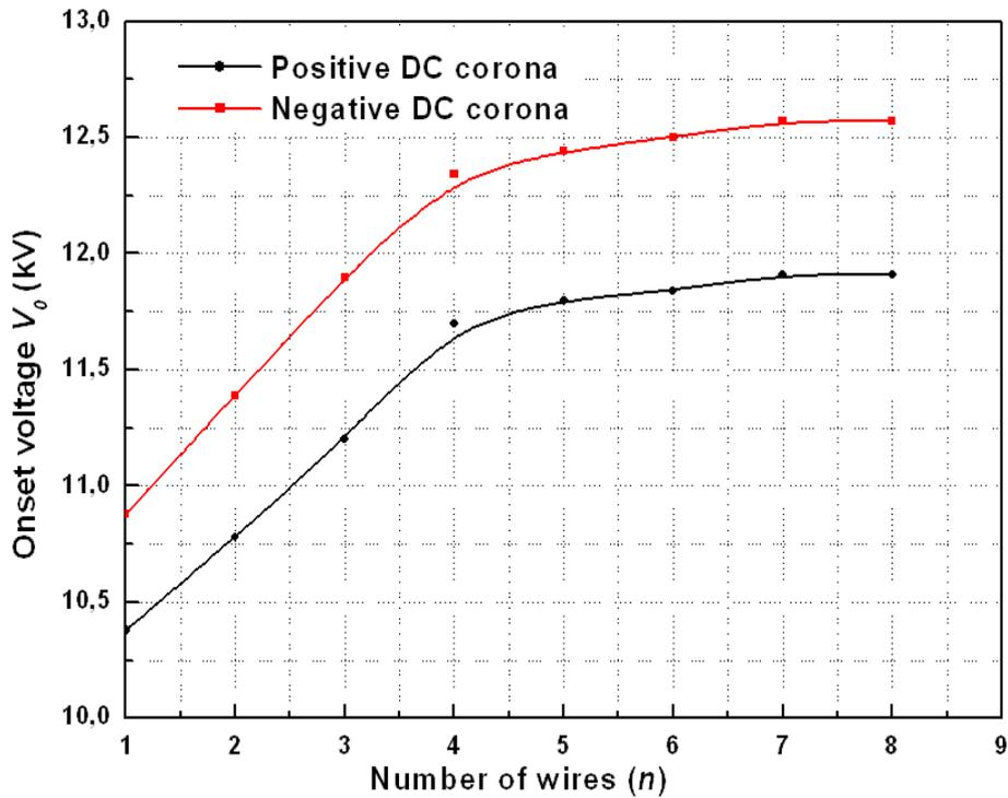
**Fig. 6.** Onset corona voltage versus the number of discharging wires.
