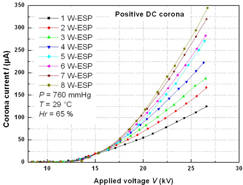
Fig. 2. Current-voltage characteristics for the DC positive corona.
