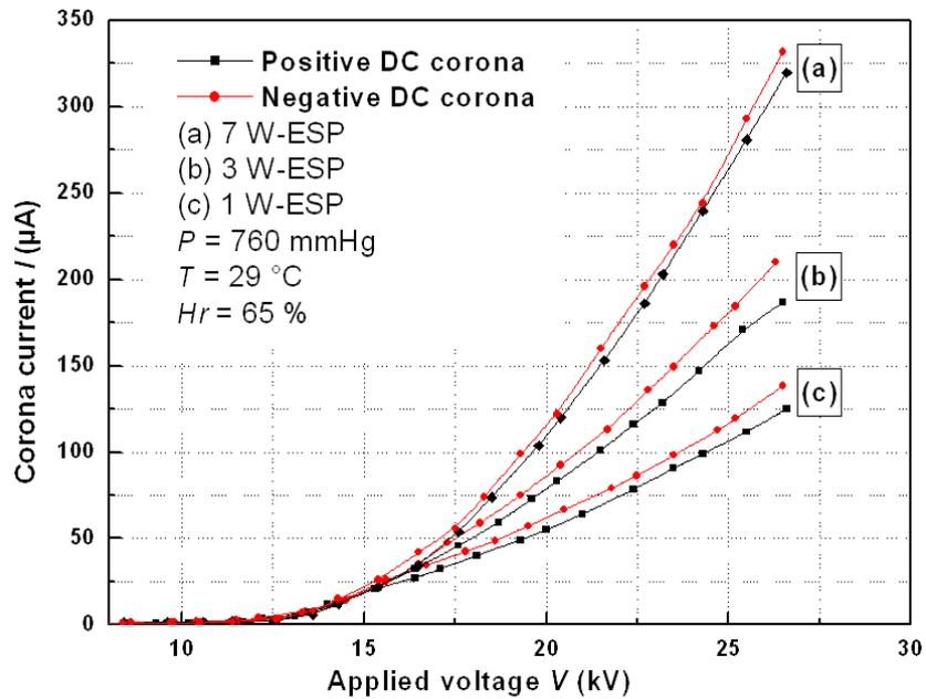
**Fig. 5.** Comparison the current-voltage characteristics for the positive and negative corona.
