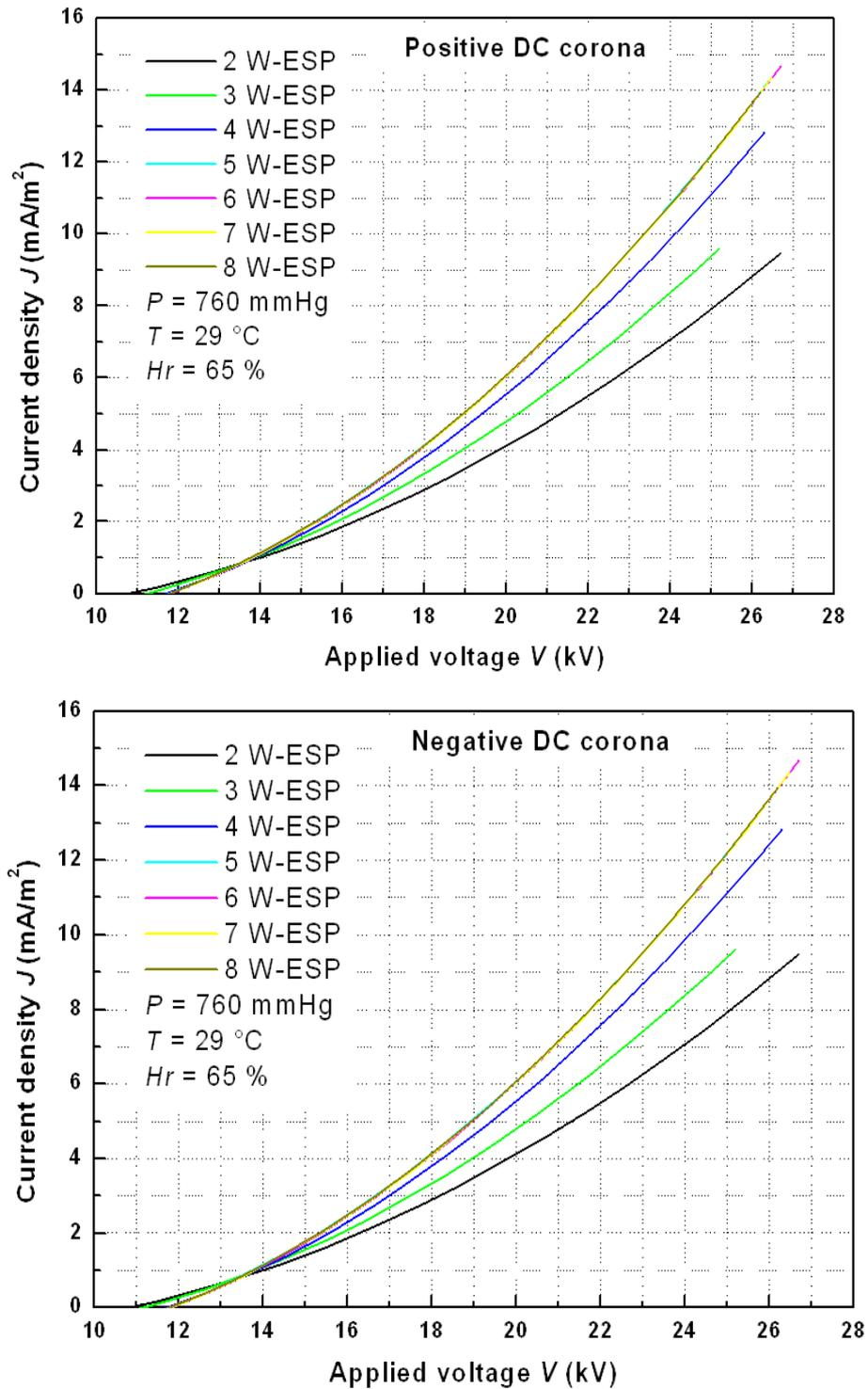
**Fig. 14.** Variation of the orona current density with the wires number.
