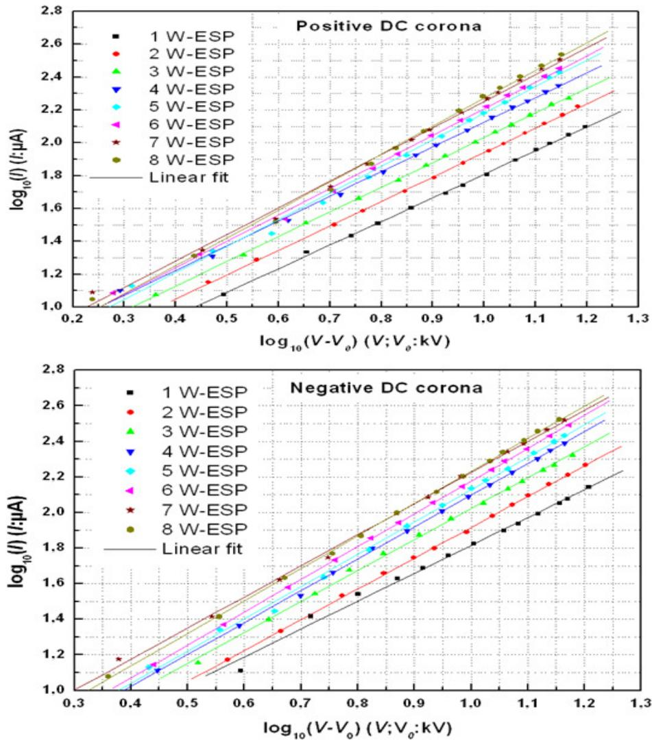
**Fig. 4.** The dependence of the current  $I$  on the voltage difference  $(V - V_0)$  on a log scale.
