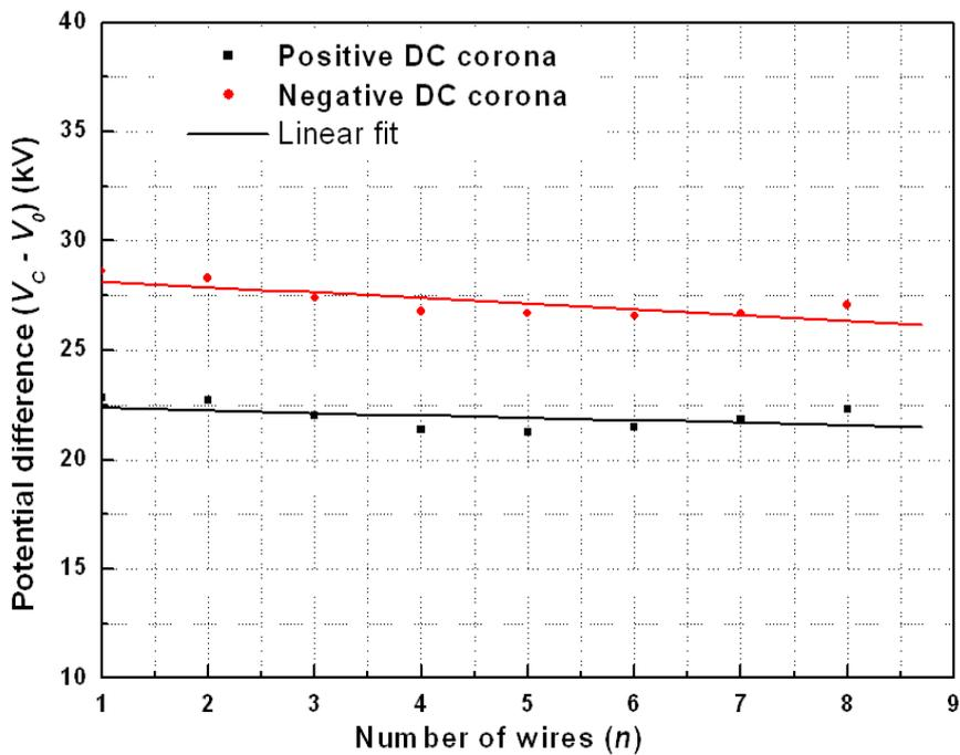
**Fig. 9.** Potential difference according to a number of wires.
