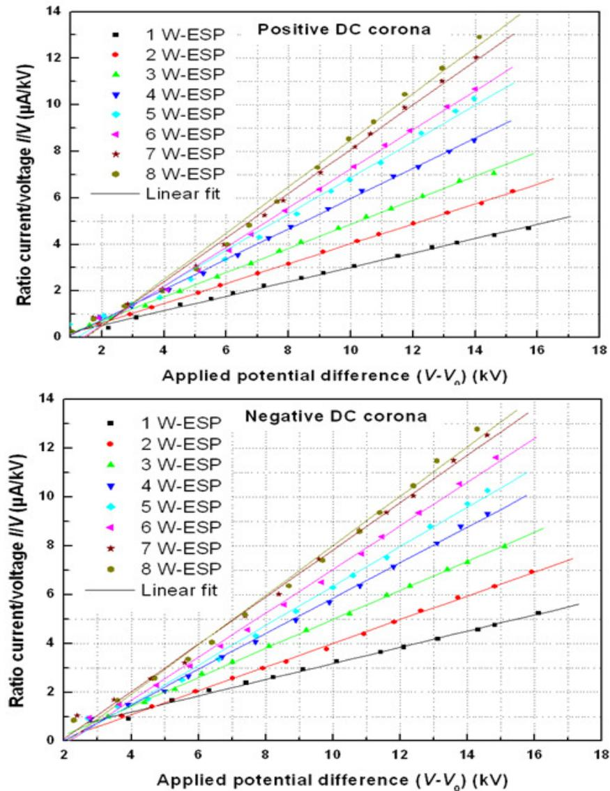
**Fig. 10.** The dependence of the current/voltage ratio ( $I/V$ ) on the voltage difference  $(V - V_0)$
