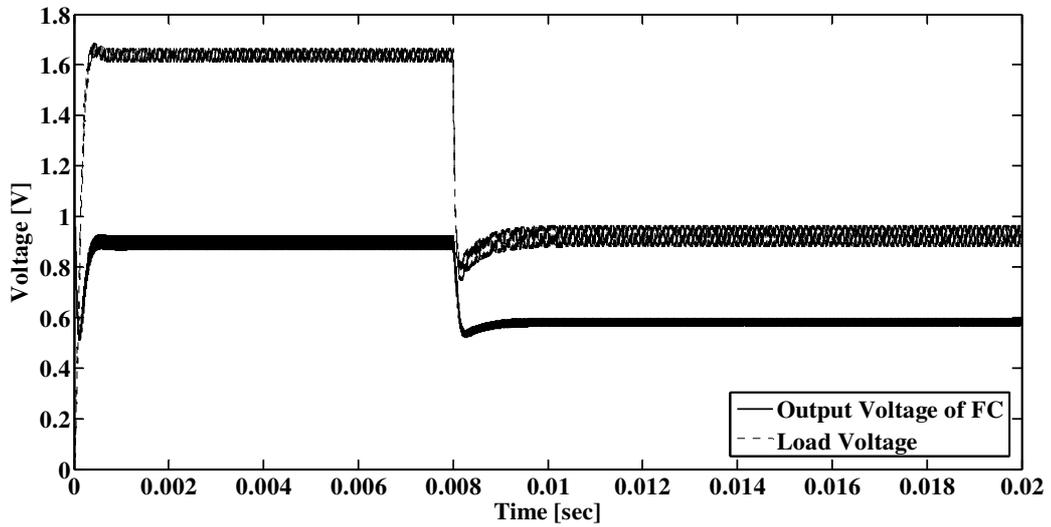
Fig.9. FC voltage and load voltage- with superconductor
