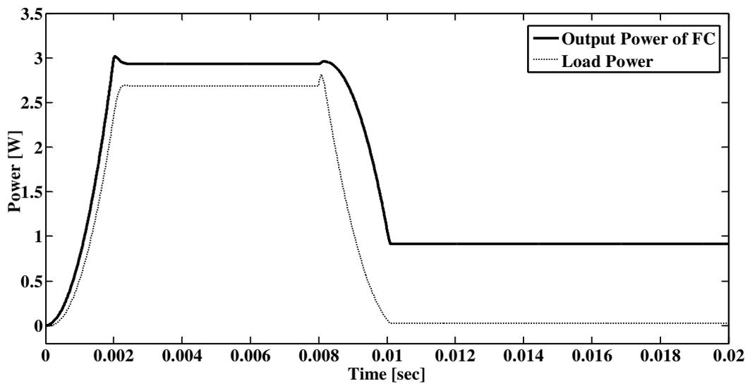
Fig.7. FC power and load power- without superconductor
