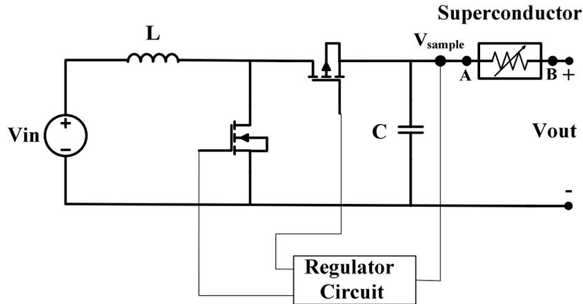
Fig.3. Proposed scheme for low-power converters
