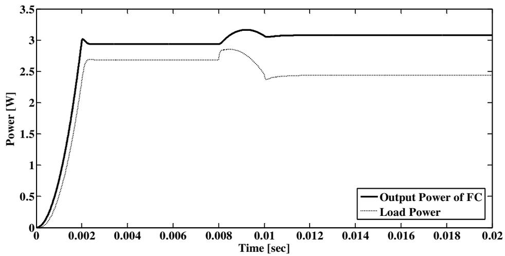
Fig.10. FC power and load power- with superconductor
