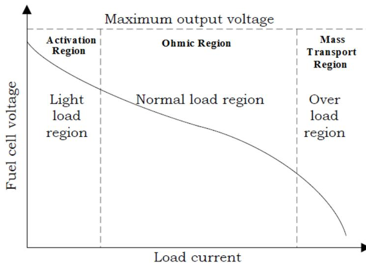
Fig.1. Polarization curve of fuel cell
