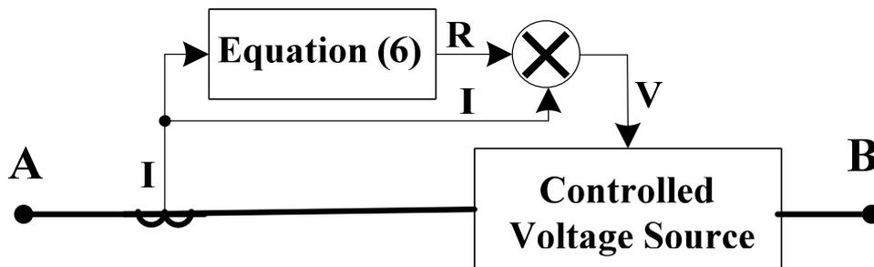
Fig.4. Block diagram of the superconductor Model
