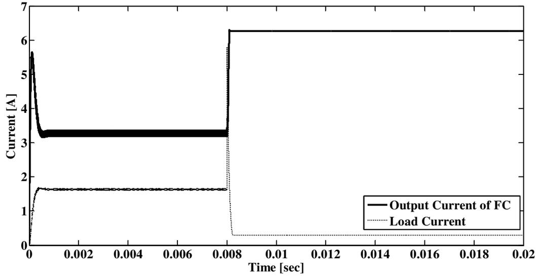
Fig.5. FC current and load current- without superconductor
