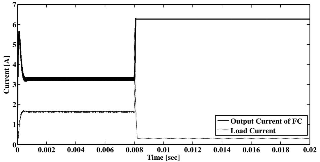
Fig.6. FC current and load current- without superconductor
