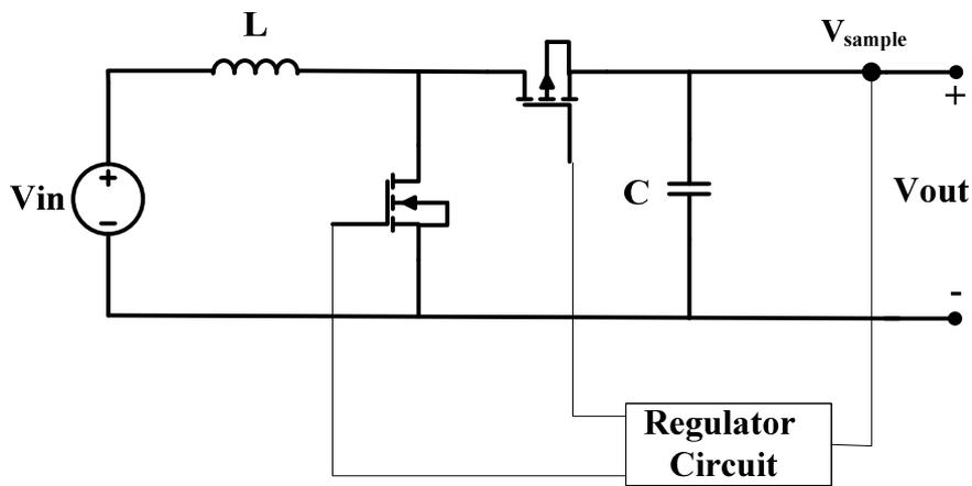
Fig.2. Circuit diagram of a DC-DC boost converter
