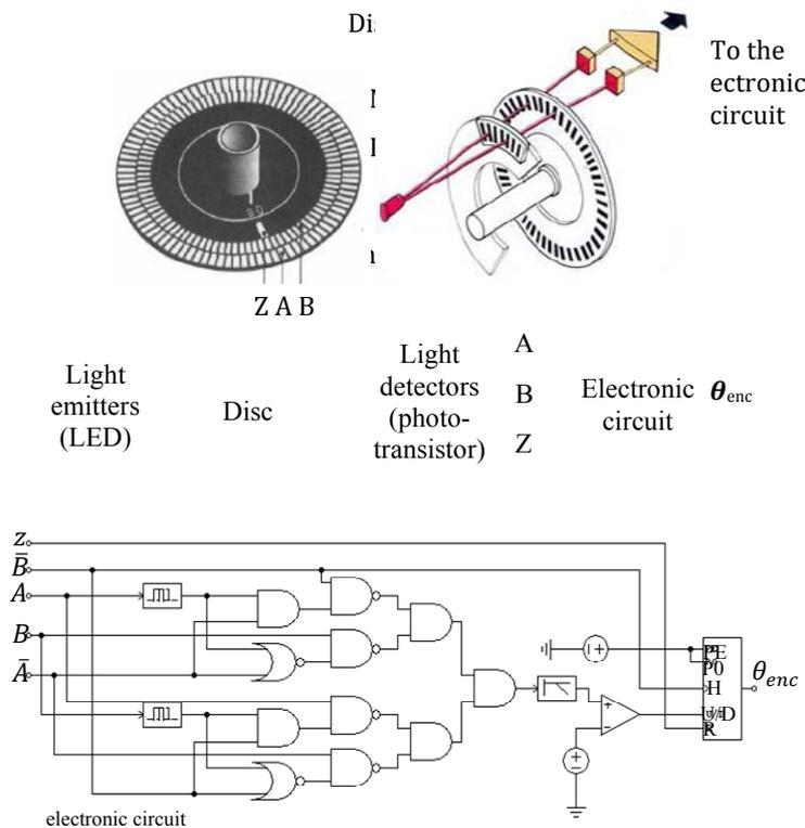
Fig. 6. Blocs diagram of the incremental encoder and electronic circuit.
