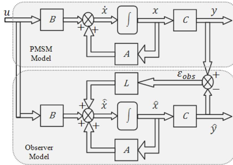
Fig. 3. Structure of the Luenberger observer.
