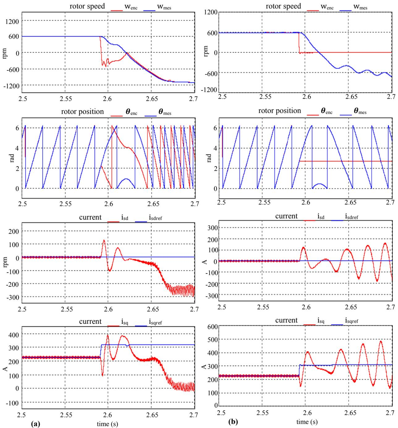
Fig.7. Simulation results in case of (a) signal A failure, (b) signal Z failure.
