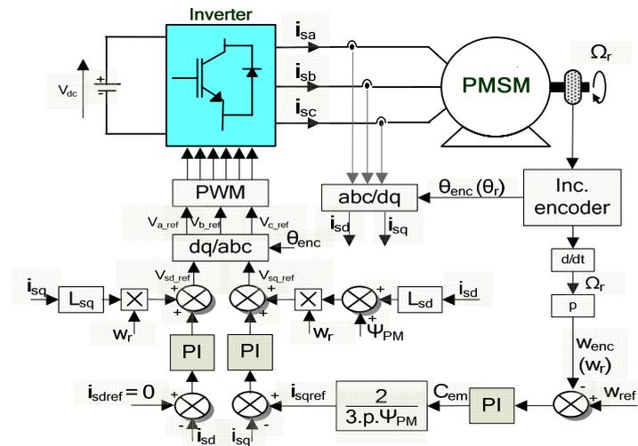
Fig.1. PMSM drive structure.
