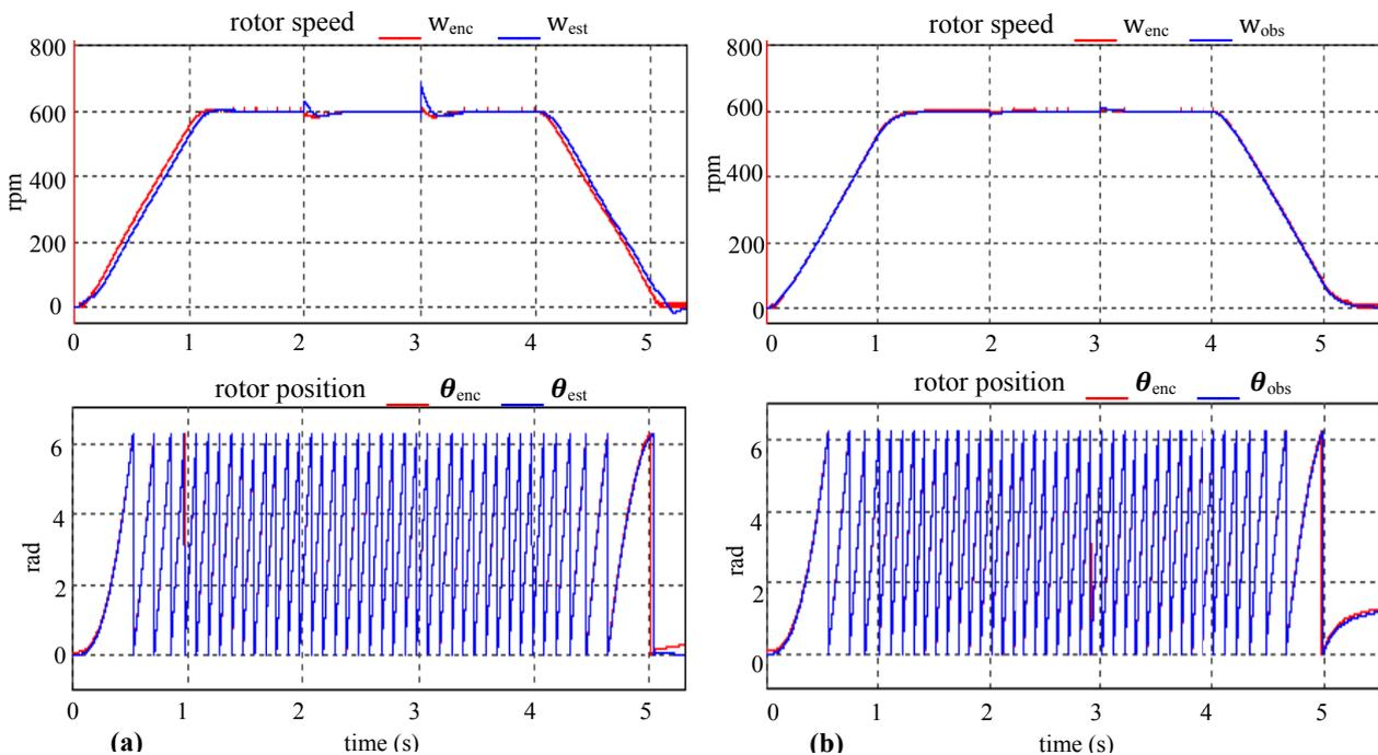
Fig.5. Speed and position in case of sensorless control using (a) MRAS estimator and (b) Luenberger observer.
