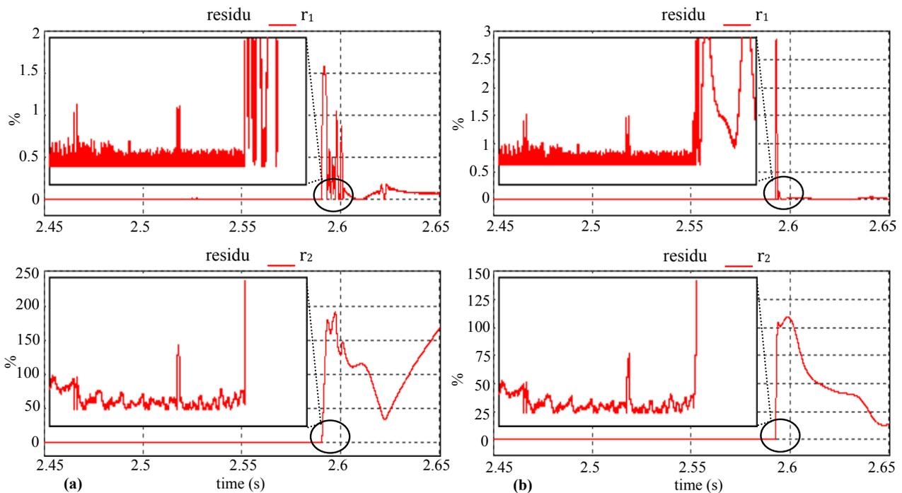
Fig.8. Residuals before and after (a) signal A failure, (b) signal Z failure.
