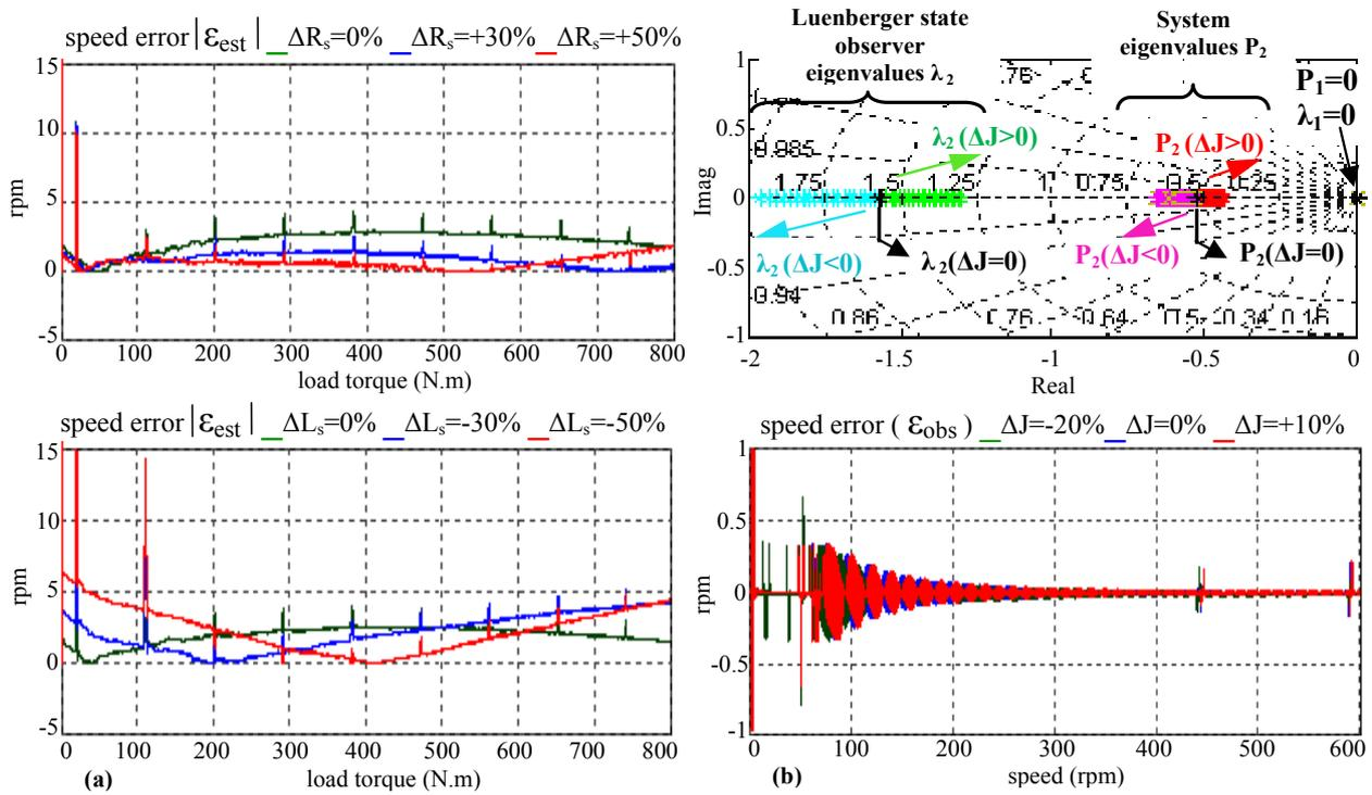
Fig.4. Robustness of the (a) MRAS estimator and (b) Luenberger observer, in case of PMSM parameters variations.
