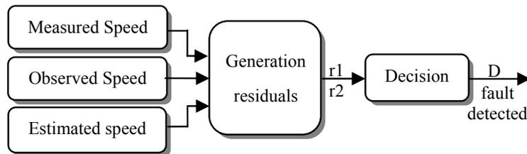
Fig.9. Technique of residual generation and detection method used.
