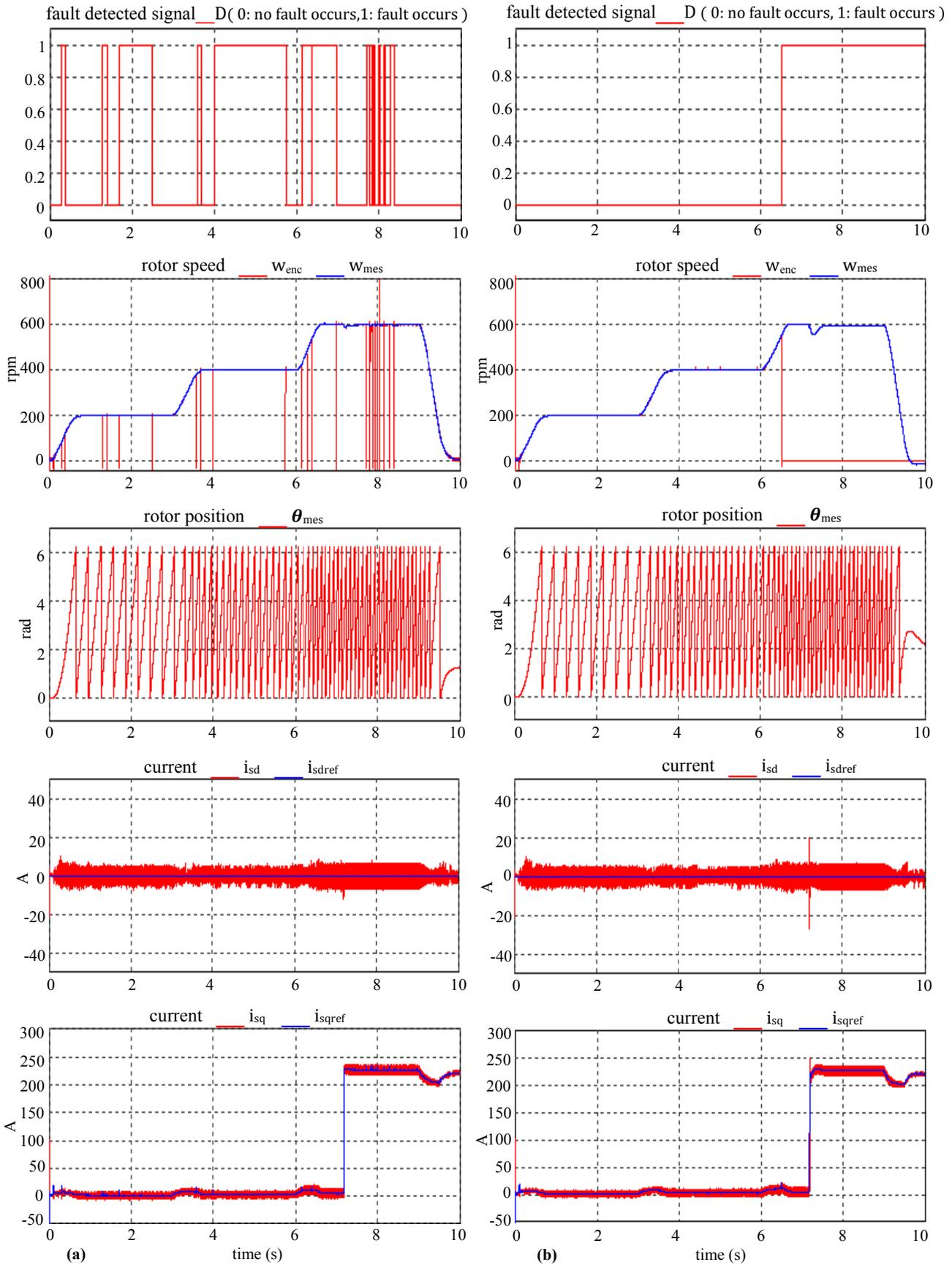
Fig.12. Reconfiguration of the system in case of (a) intermittent signal A connection, (b) permanent signal Z failure.
