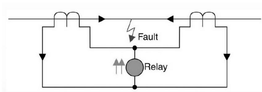
Figure 3. The structure of the differential protection
