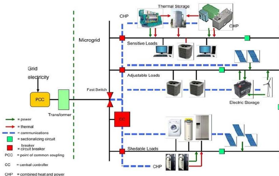
Figure 1. The configuration of a typical micro-grid
