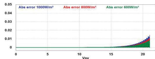
Fig. 12. Absolute errors between the I-V curve generator using table and mathematical model for different irradiances
