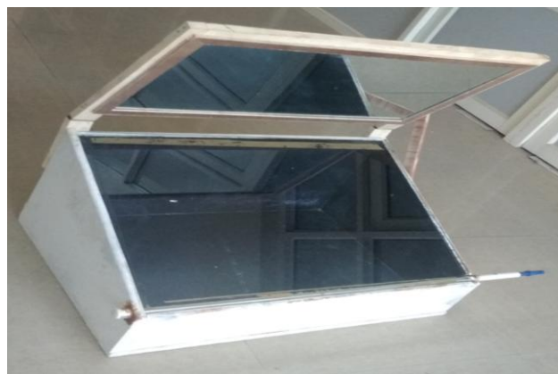
Figure 2: Solar water distillation with using reflector
