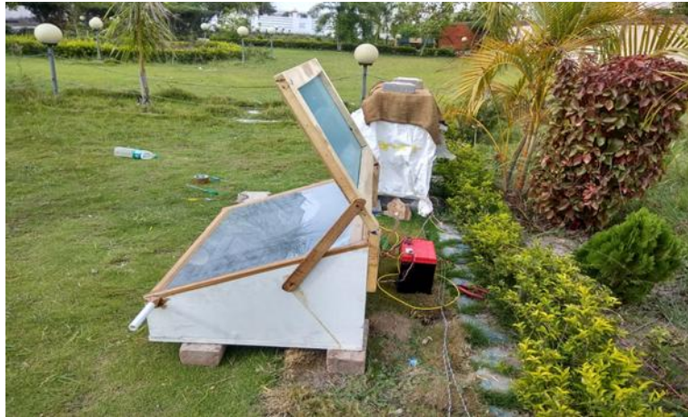
Figure 5: Solar Water distillation with Heating element powered by Solar PV
