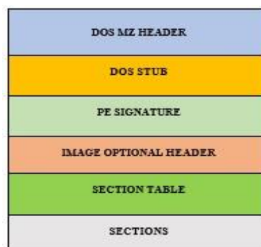
Figure 1. The PE file's fundamental structure.
