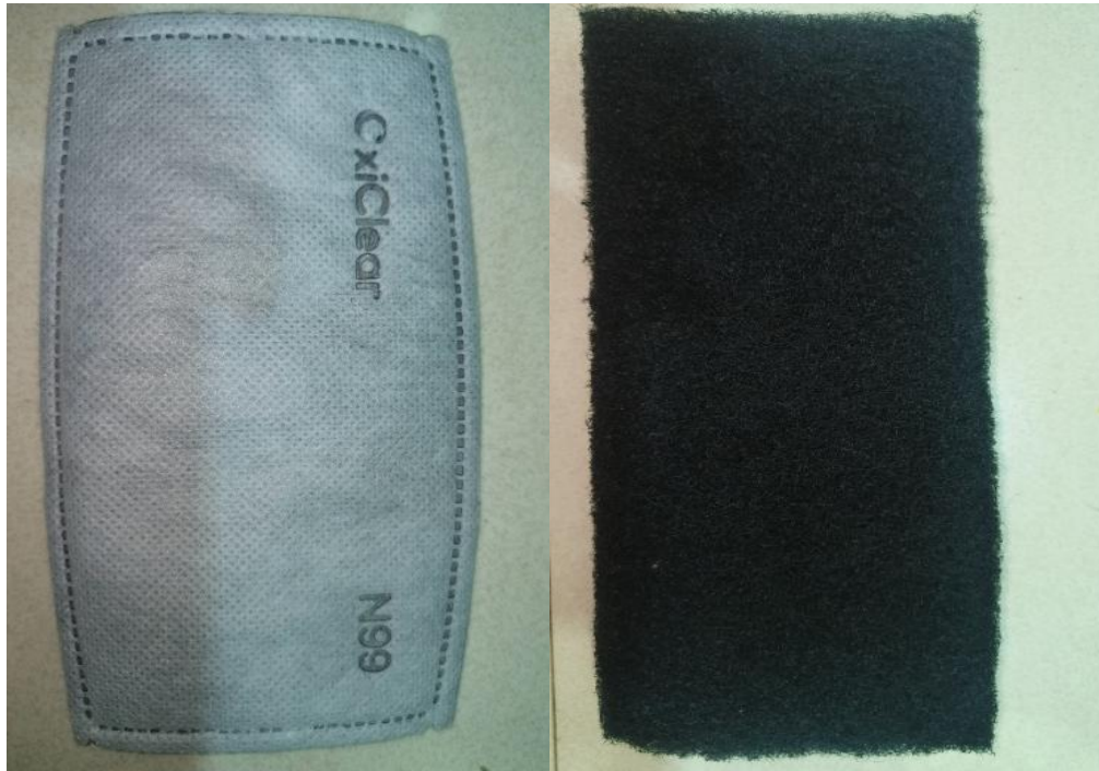
Fig.6. Activated Carbon Filter and Activated Carbon Foam Filter
