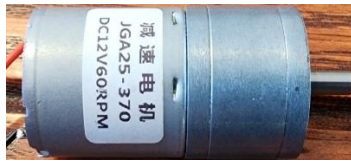
Fig. 5. Geared DC Motor drives
