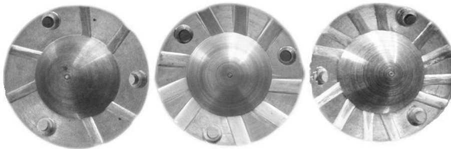
Fig. 2: TWO, THREE AND FOUR NUMBER OF GROOVES ON THE BRASS CROWN PISTON
