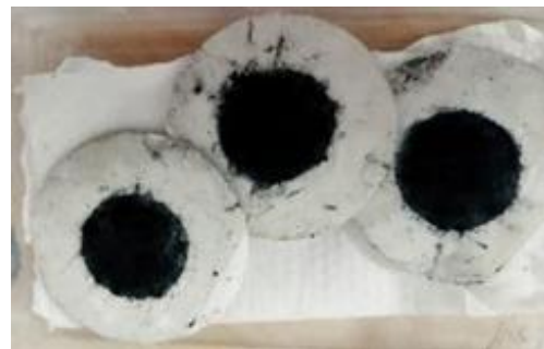
Figure 2: Solution coated onto the electrode
