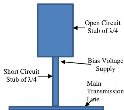
**Fig.1. Layout of Loaded Line Phase Shifter**
