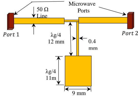
**Fig.2. Layout of Loaded Line Phase Shifter using CST**
