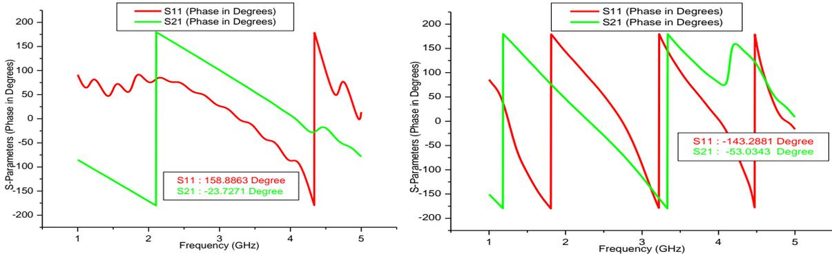
**Fig. 3. S-Parameters S11= -153.88° and S21= -23.72° without LLPS (Left) and S11= -143.28° and S21 = -53.03° with LLPS (Right)**
