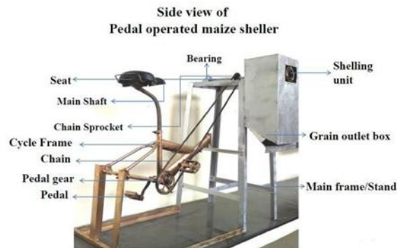
Figure.2 Side view of pedal operated maize sheller
