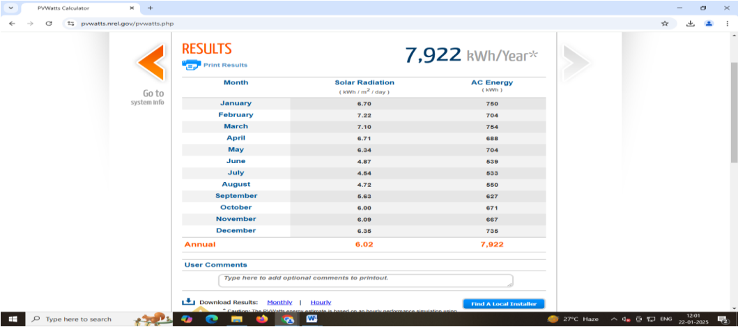
Fig.4 Simulation results of 5KWp Solar rooftop plant
