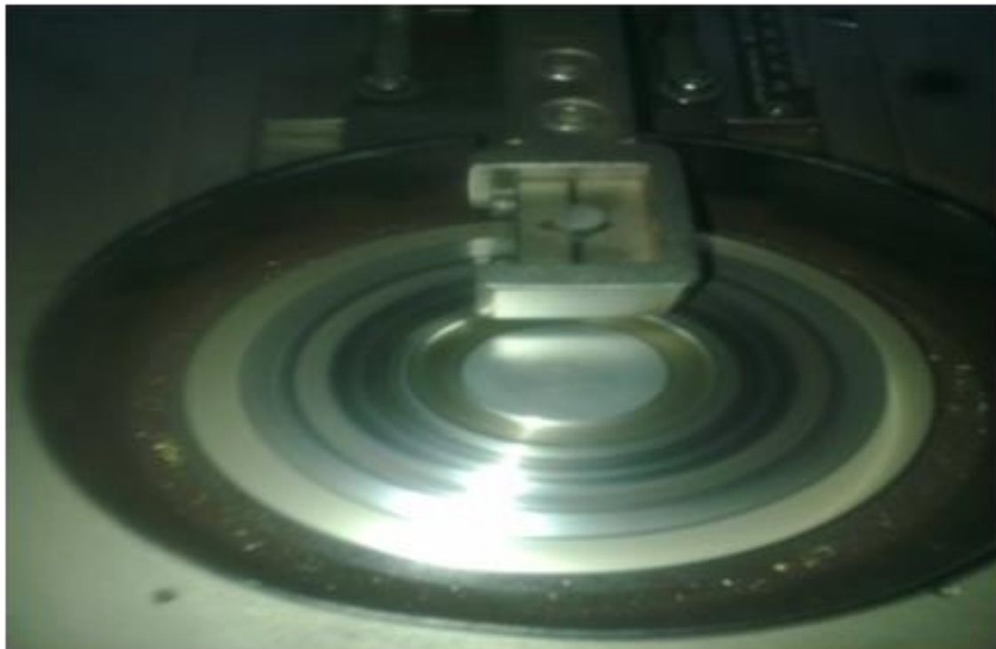
(a) Carbon steel disc with pin fitted into it
