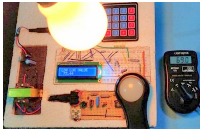
Fig. 9. Shows the lux value for both the sensors (reference lux meter and LACFSOC) at a 30% power cycle.
