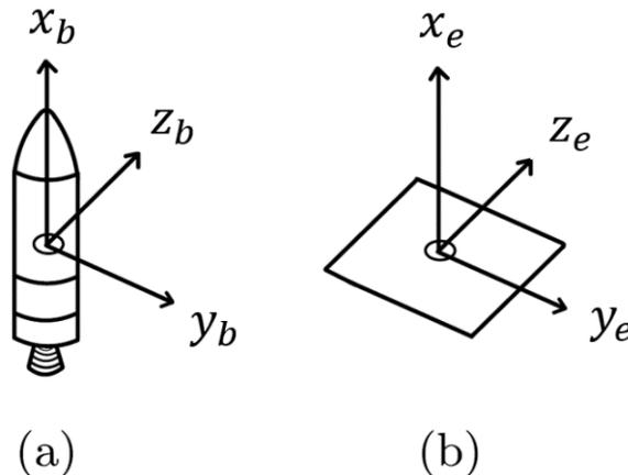
Fig. 1 (a) Body-fixed and (b) inertial reference frames
